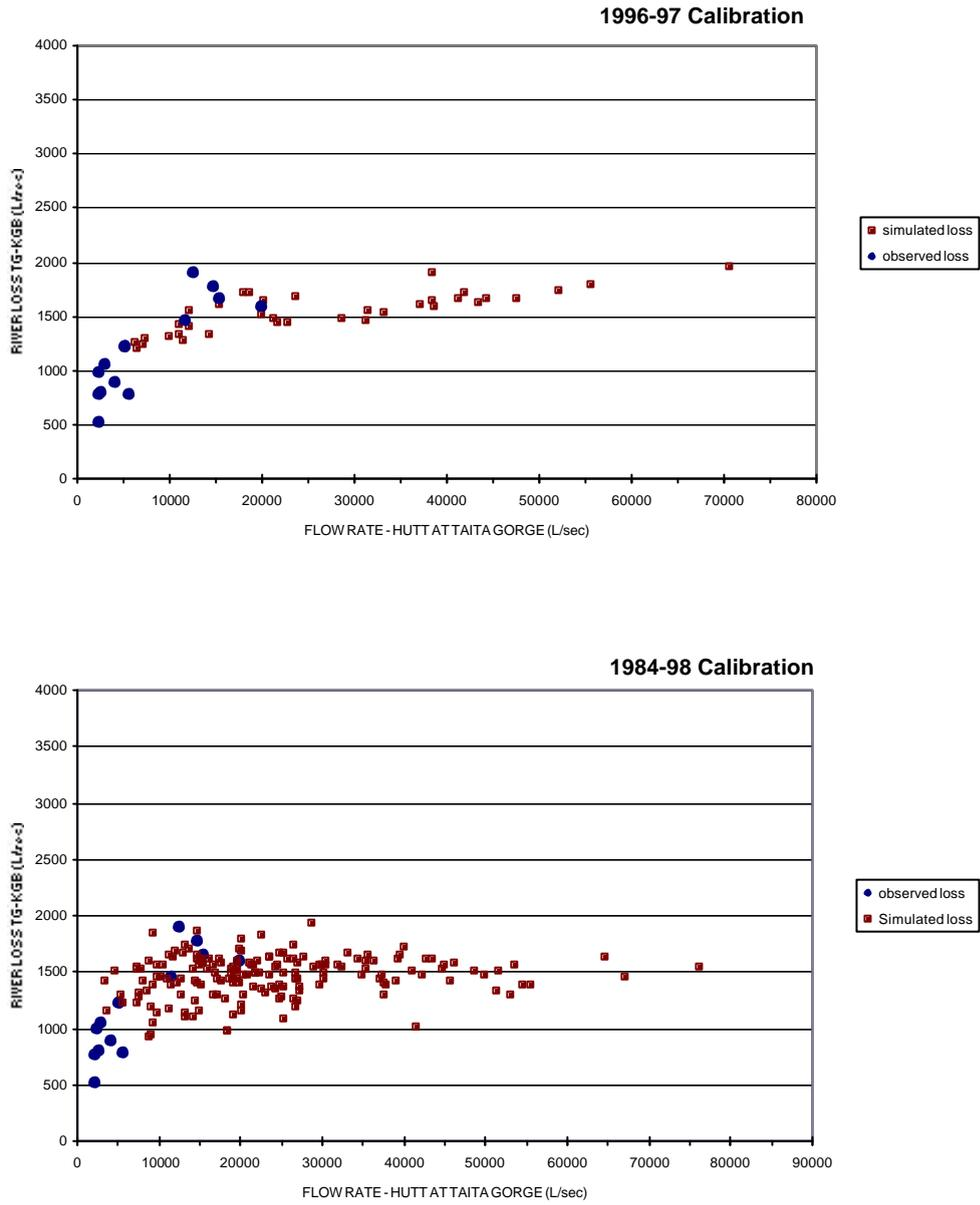
Figure 14 : Model calibration – simulated river bed losses vs flow at Taita Gorge
