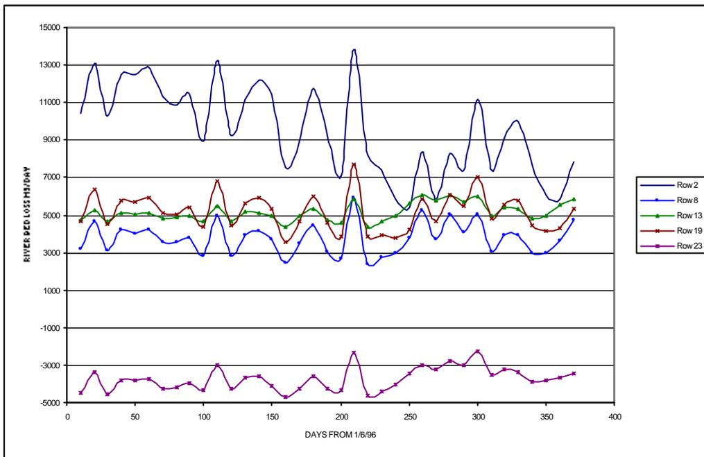
Figure 13 : Simulated river bed losses at selected model rows.
