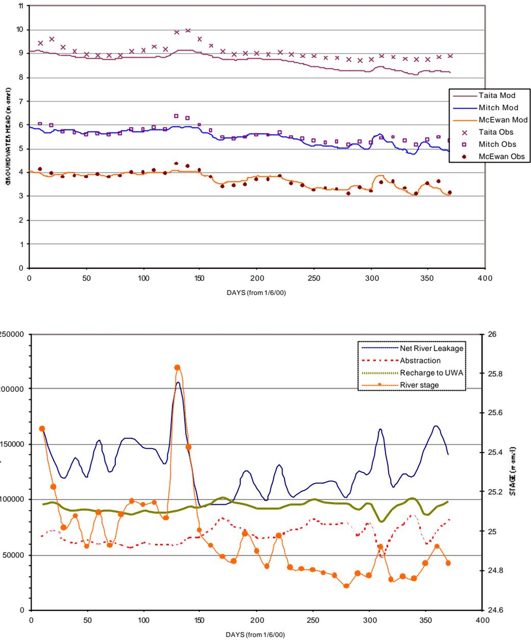
Figure 16 : Transient calibration verification
