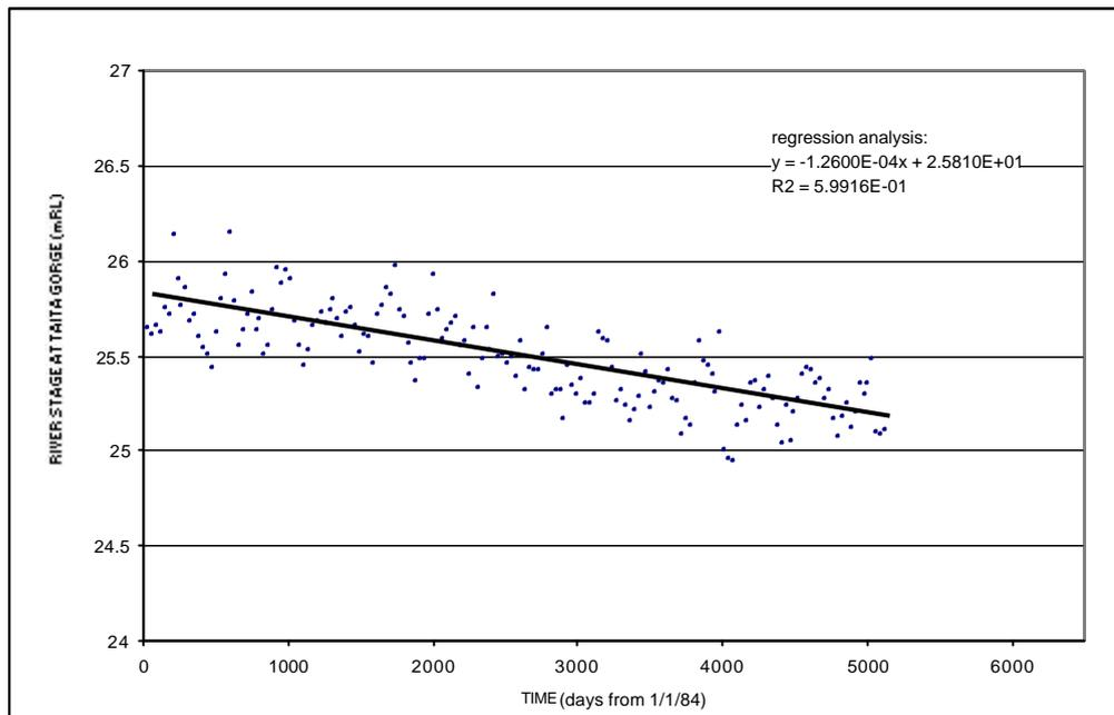
Figure 8 : Long-term change in Taita Gorge stage associated with bed level degradation.
