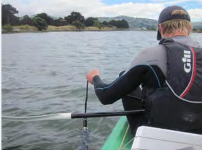
YSI data sonde recording water quality parameters of DO, salinity, chl-a, depth and temperature.
