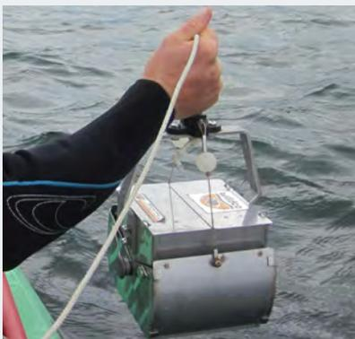
Box core being prepared for deployment (photo above), and retrieved after sample collection (photo below).
