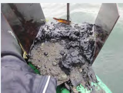
Purpose built shallow water sediment sampler for collecting coarse sediments. Note the ability of the corer to retain unconsolidated organically enriched surface deposits overlying clean bottom sediments.
