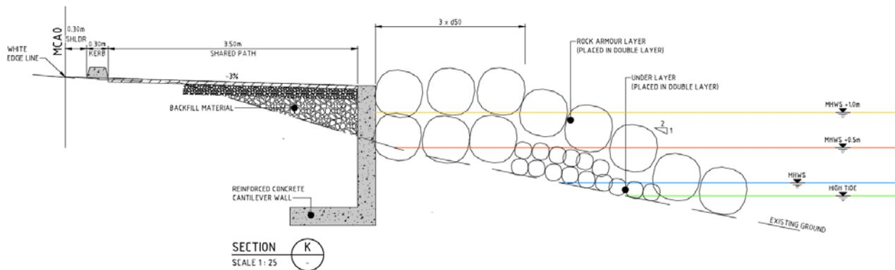
Figure 3-1: Typical revetment with reinforced concrete cantilever wall
