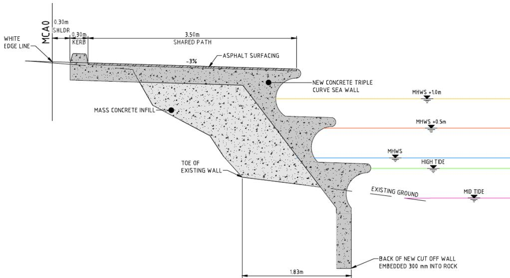
Figure 3-5: Triple curved concrete wall
