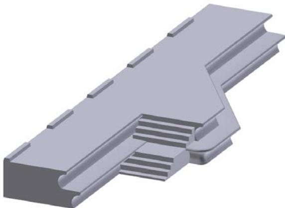
Figure 3-6: Parallel Access Steps on Double Curve Wall
