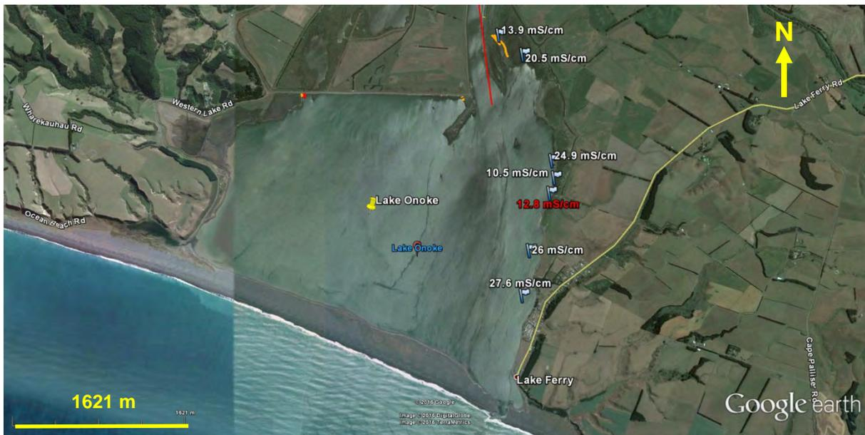
**Figure 22b.** Conductivity of waters in Lake Onoke illustrating the lower readings in the vicinity of freshwater seeps along the north and eastern shoreline. Red line = Ruamahanga River course. Red value is conductivity in an occluded lagoon formed by a historic old braid, separated from the lake by a gravel bund.
