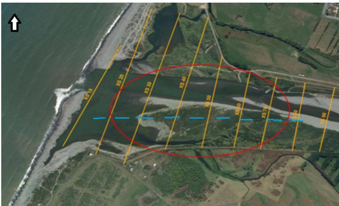
Figure 14: Location of the area known as ‘Mangahanene Island’ (circled in red) with approximate position of design channel on left bank shown in blue
