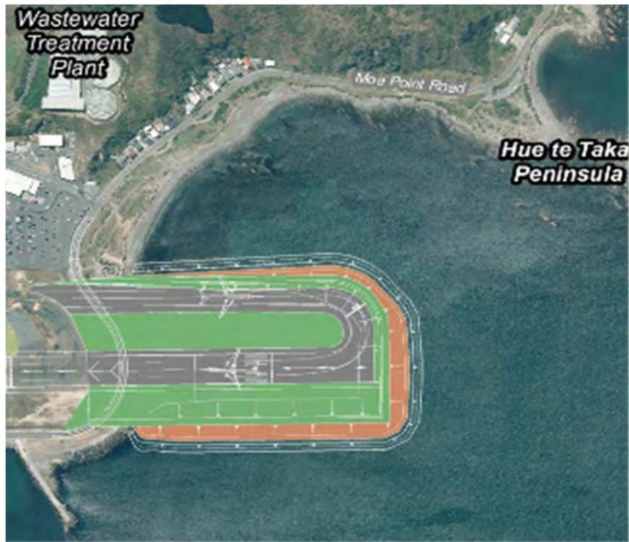
**Figure 5:** Part of Figure 1, ALVE, illustrating relative surface areas of the runway extension and the residual area of the Moa Point embayment. The area of sea to be reclaimed for the runway extension appears at least as great, if not greater, than the adjacent sea surface area that will remain within the embayment, post-construction. Note also the acute angle created between the embayment beach and the extension (Source, Figure 1, Site Context, ALVE report)
