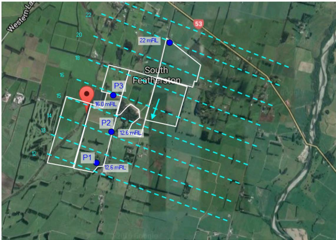
**Figure 3** Interpreted Piezometric Surface Map
