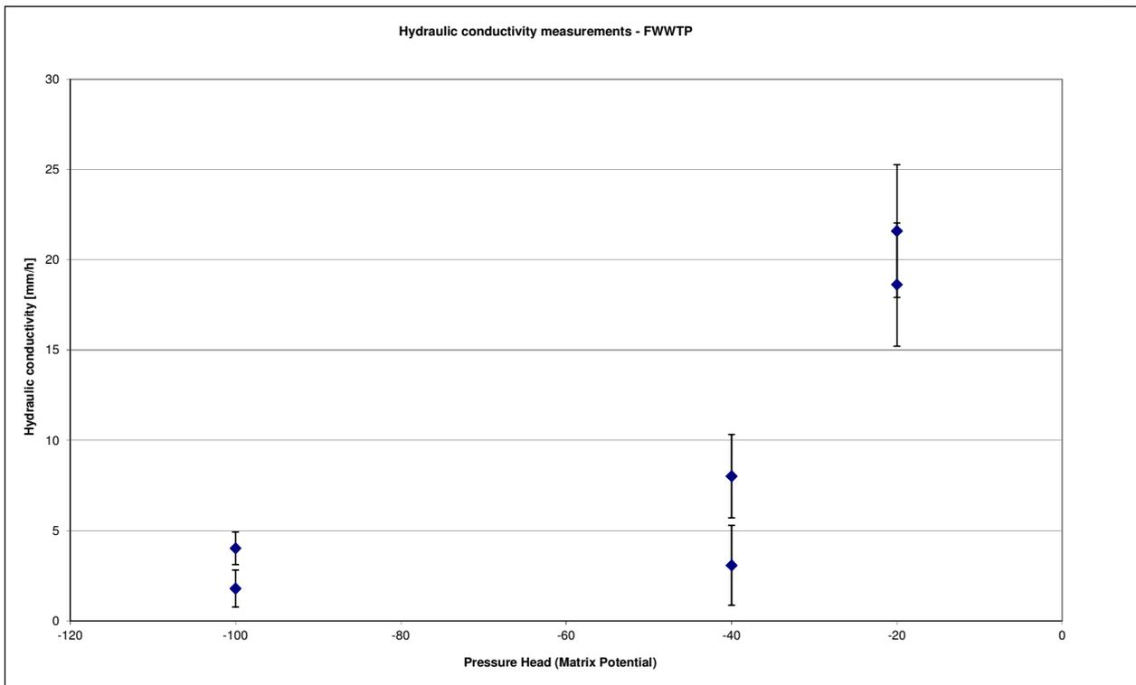
**Figure 5.1: Unsaturated Hydraulic Conductivity – FWTWTP Site**
