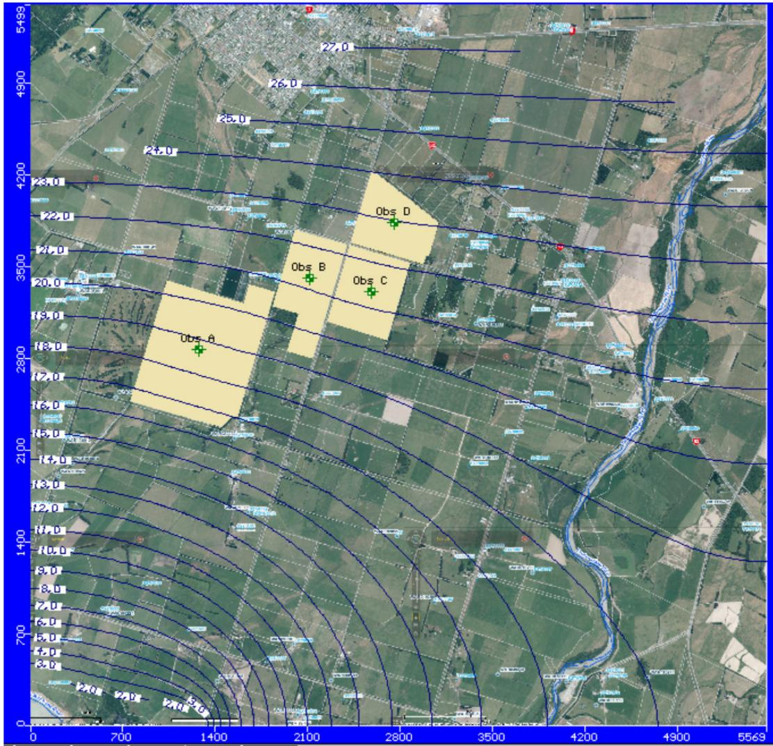
**Figure 2 MODFLOW Steady State Head File**
