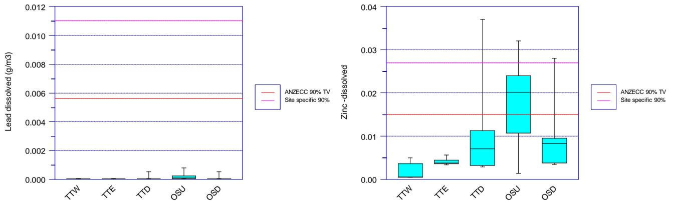
Figure 3-13: Dissolved lead and zinc by site compared with TV's (2010 - 2016)
