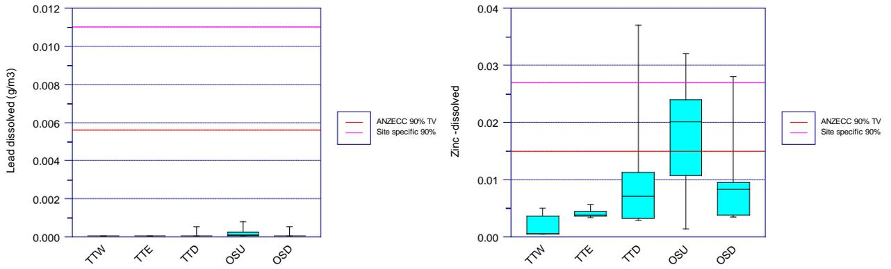
Figure C-11: Dissolved lead and zinc by site compared with TVs (2010 - 2016)
