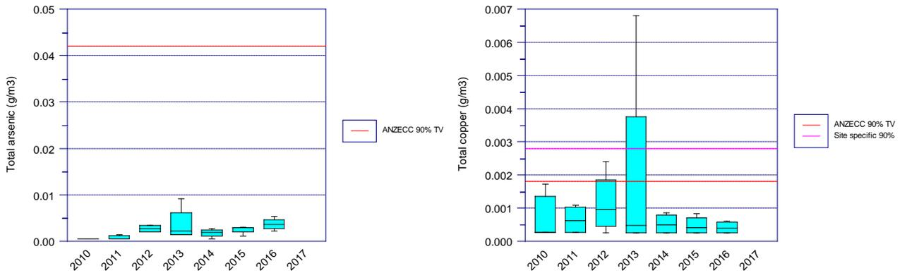
Figure C-7: Total arsenic and copper by year at site TTD
