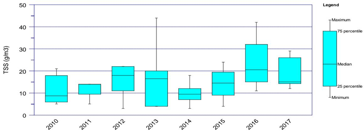
Figure C-15: Total suspended solids results by year at site TTD
