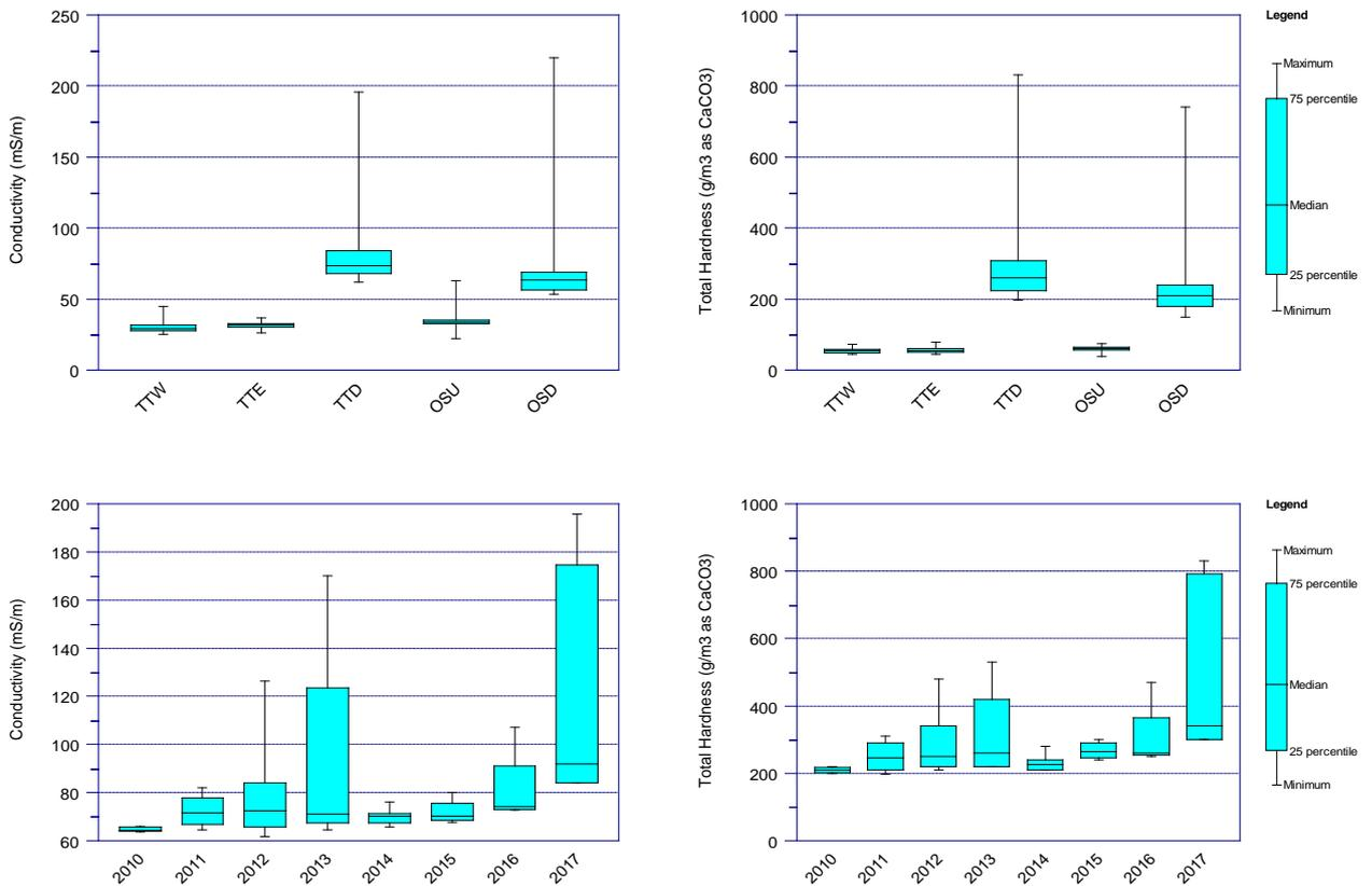
Figure C-2: Summary of conductivity hardness by site (above) and by year at TTD (below)
