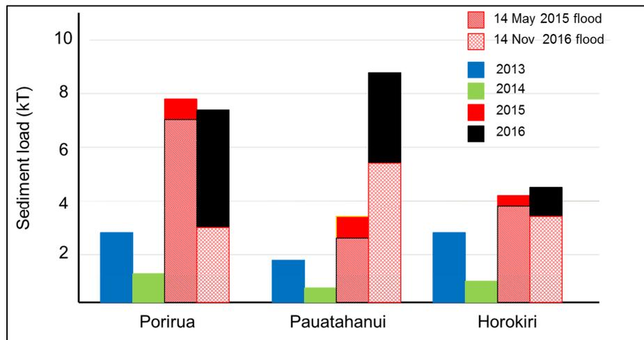
**Figure 1: Monitored sediment loads since 2013, including the two storm events in 2015 and 2016, for the three largest catchments in Te Awarua-o-Porirua.**
