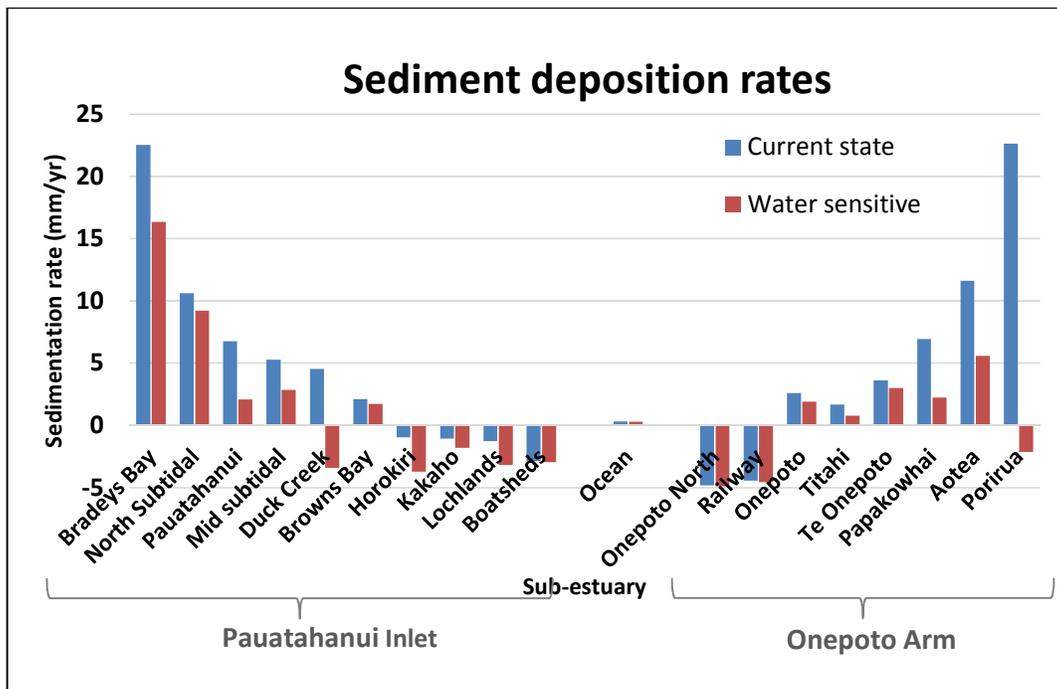
Figure 2: Sub-estuary sediment rates showing erosion and accumulation for both current state and water sensitive scenarios. Negative rates are erosion, positive rates are accumulation.
