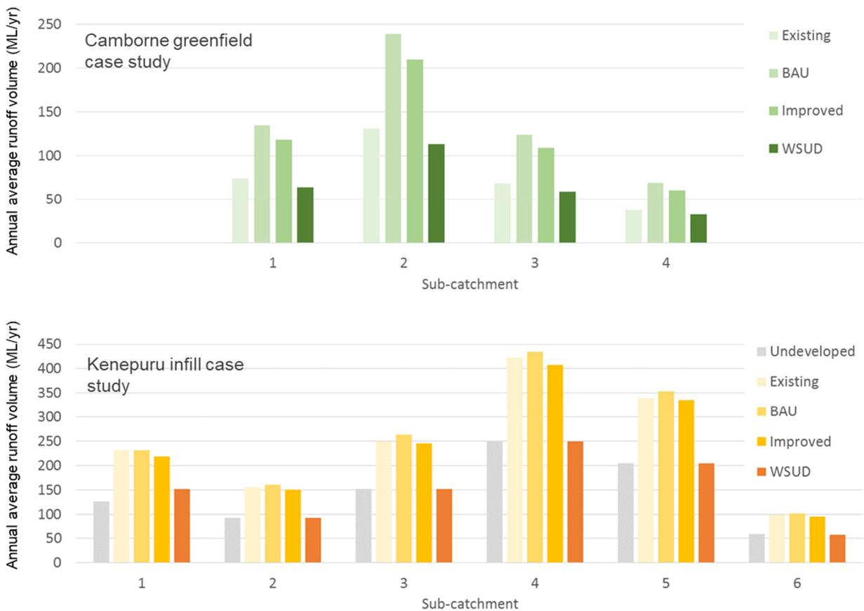
Figure 3. Changes in annual average runoff volume in each case study. Each group of bars are results for sub-catchments within each case study area. An 'undeveloped' volume has also been estimated for reference in the Kenepuru case study.
