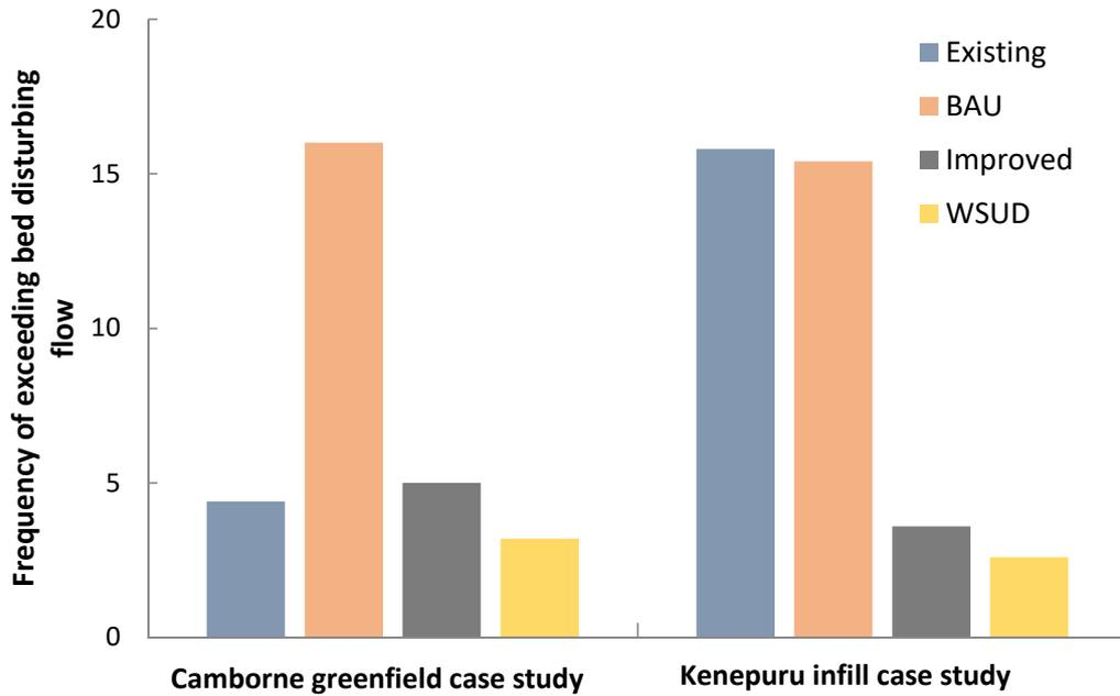
Figure 2. Changes in frequency of exceeding bed disturbing flows in each case study
