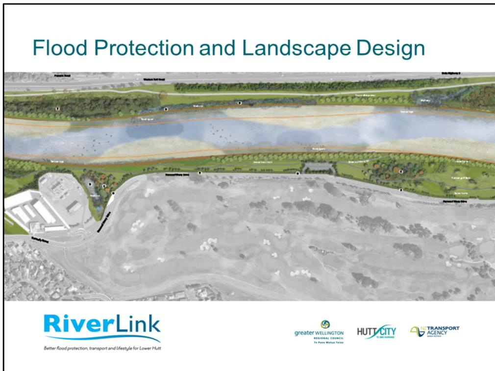
Channel capacity increased from around 75m to 110m, also removing built up gravel as part of this, and will have ongoing extraction of about 15,000 m<sup>3</sup> per year to keep it around same bed level
