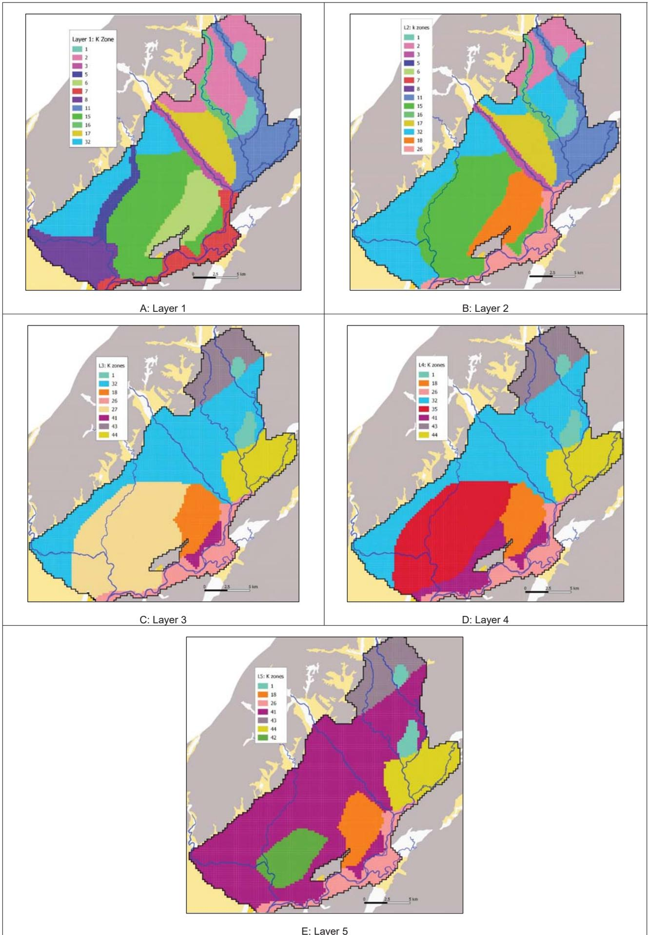
Figure 3.7 Hydraulic conductivity zonation for the northern model (numbers = zone identification numbers)
