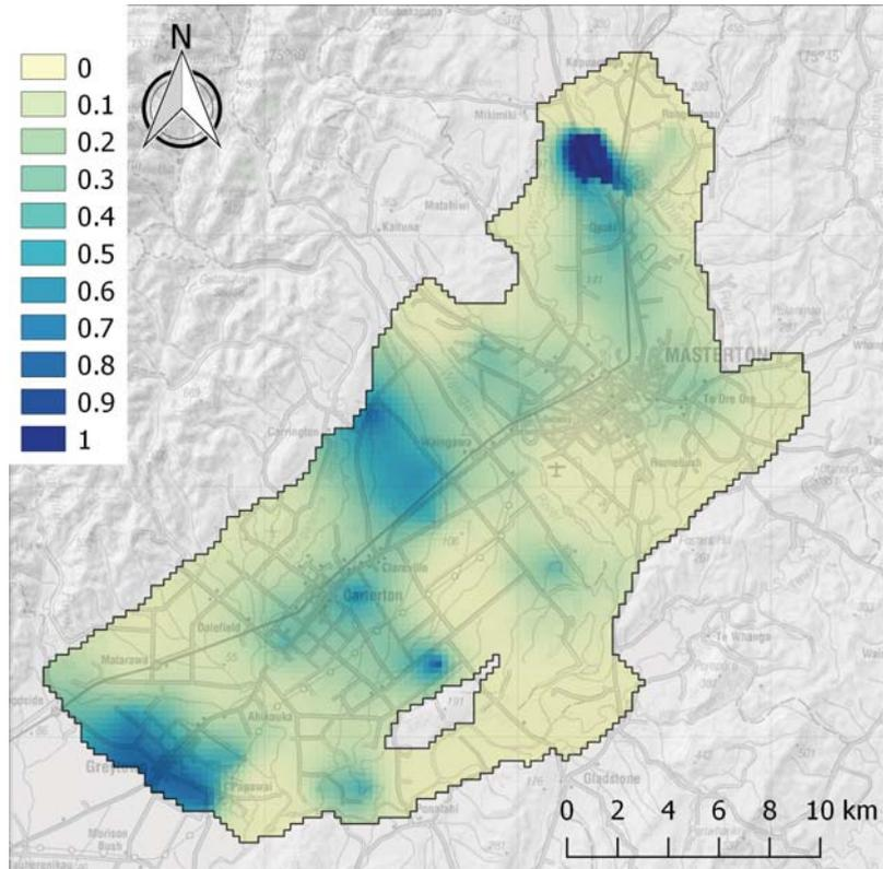
Figure 6.12 Relative parameter uncertainty variance reduction of recharge multiplier in the north model.
