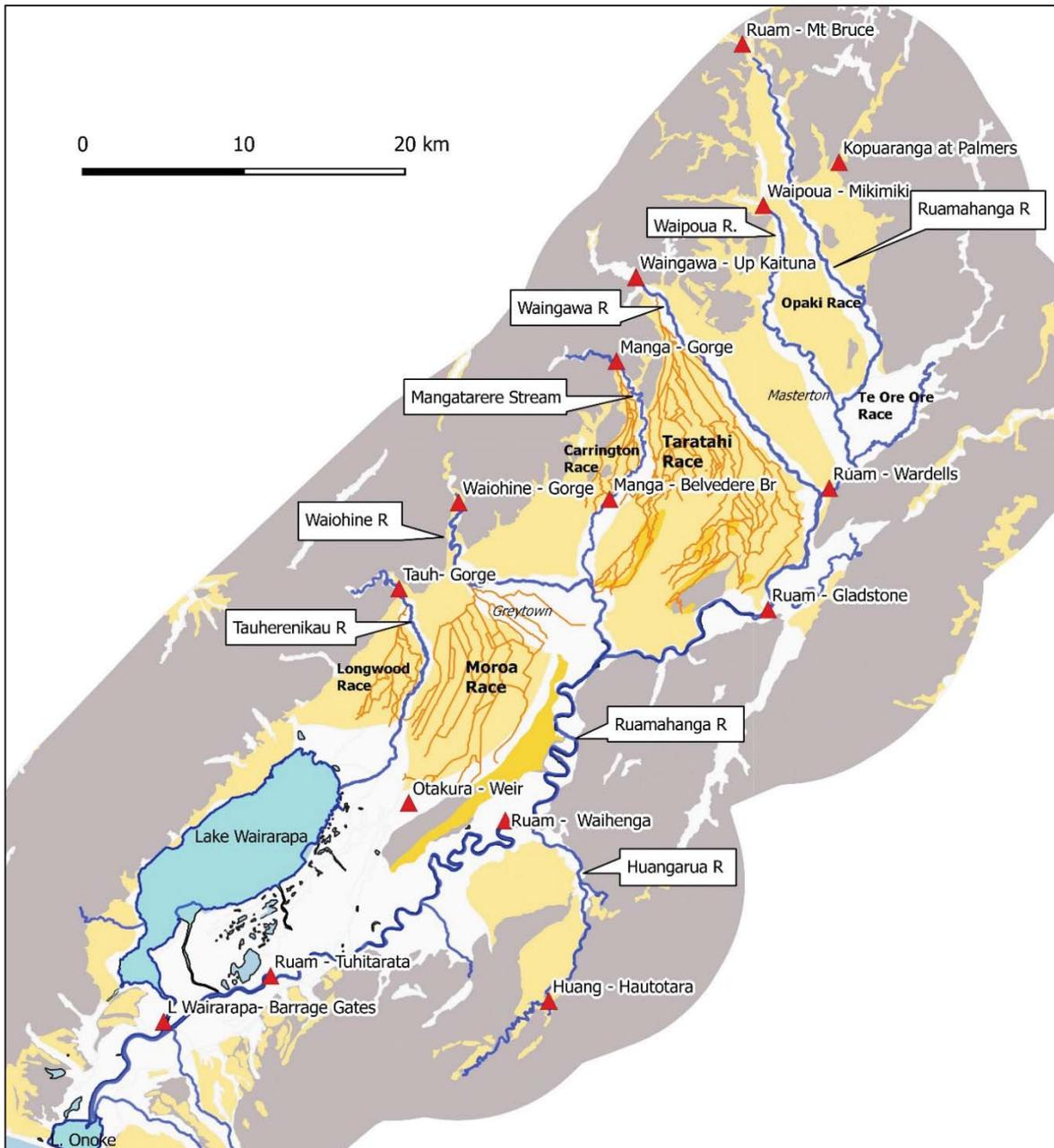
Figure A2.1 Wairarapa Valley natural drainage system — principal rivers, streams and lakes. Surface water gauging sites (red triangles) and water race networks (orange network) also shown.
