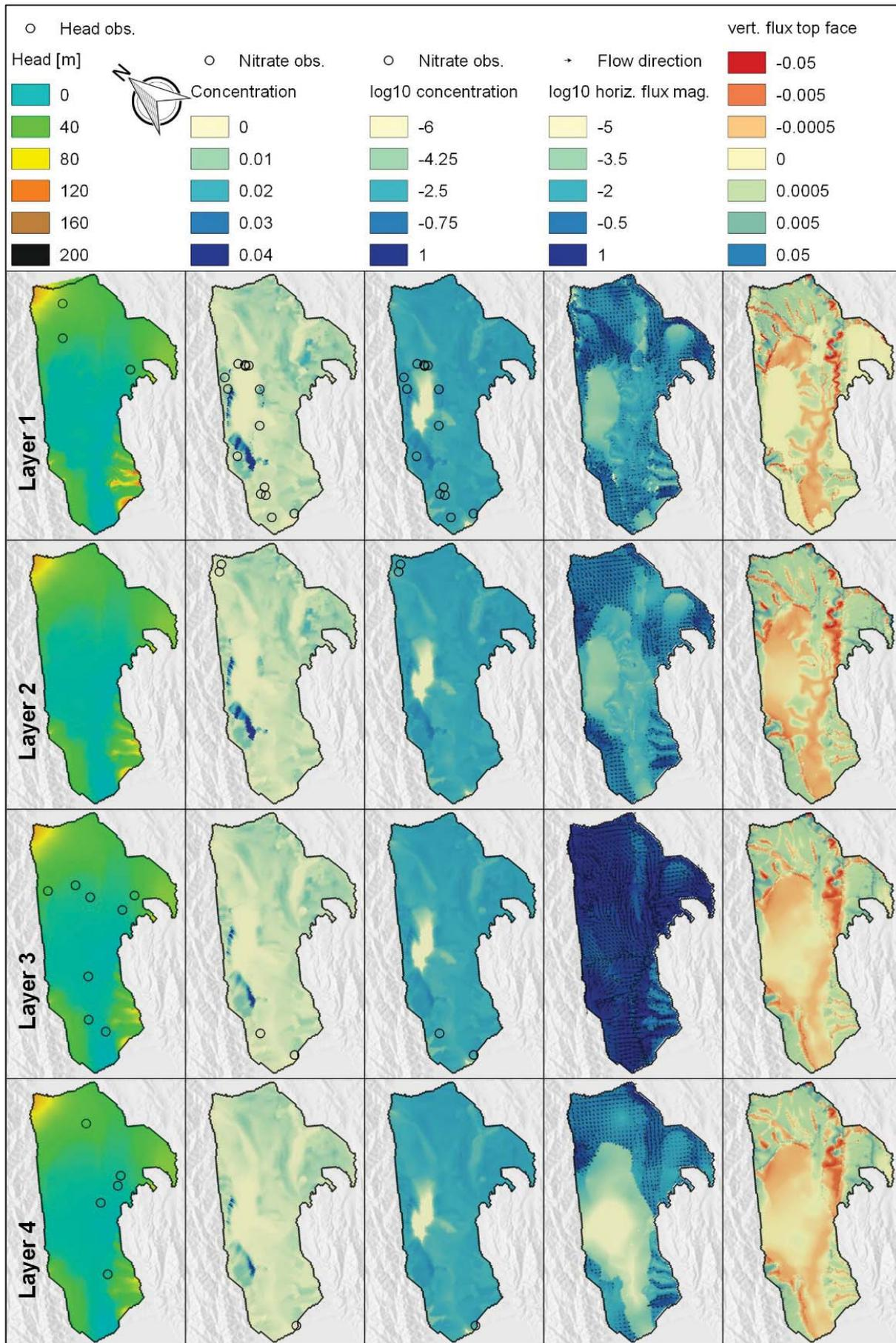
Figure 5.7 Calibrated piezometric, concentration and flux model outputs from the south model calibration (layers 1-4).
