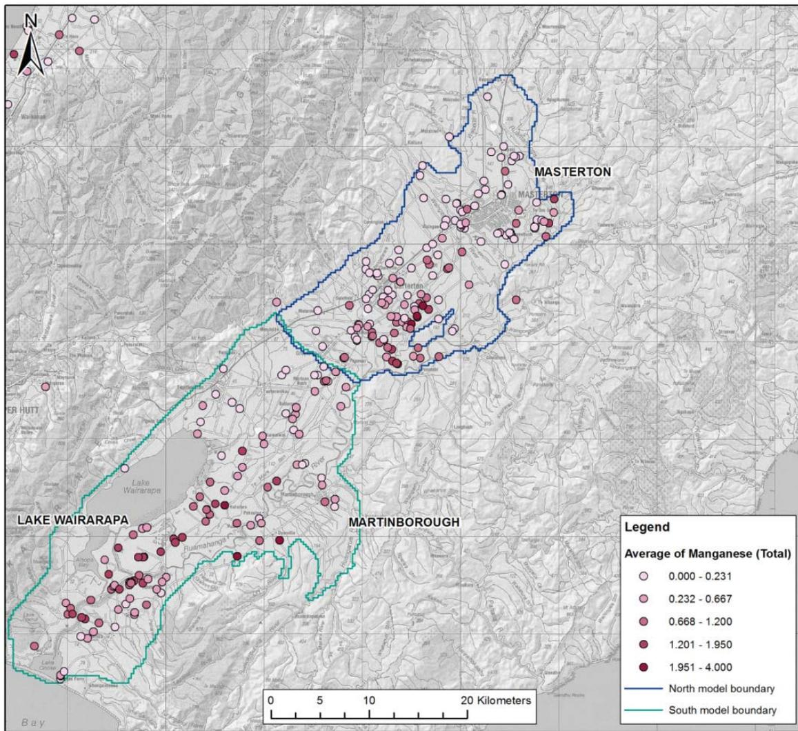
Figure 4.6 Groundwater total manganese concentration distribution in the Wairarapa Valley.
