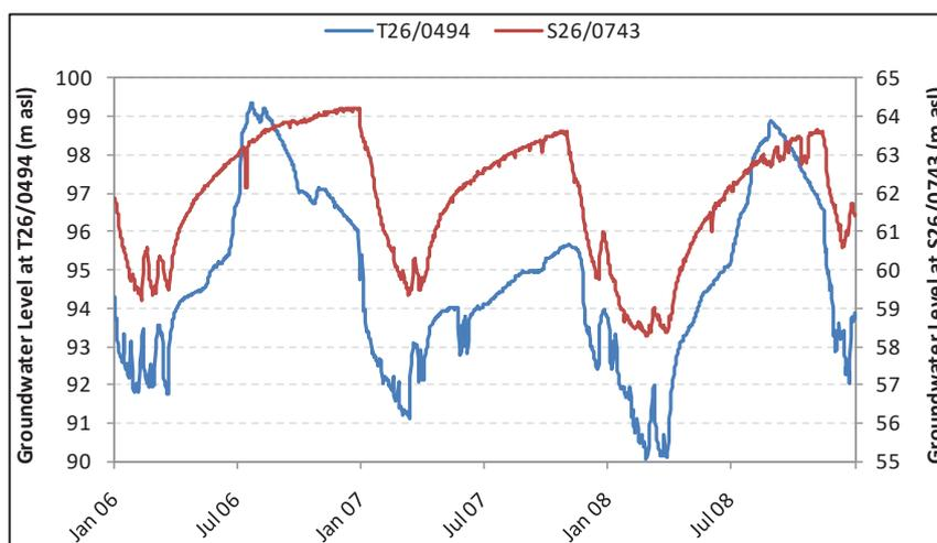
Figure A4.13 Groundwater levels in semi-confined aquifers in the Te Ore Ore (bore T26/0494) and Parkvale (bore S26/0743) alluvial sub-basins.
