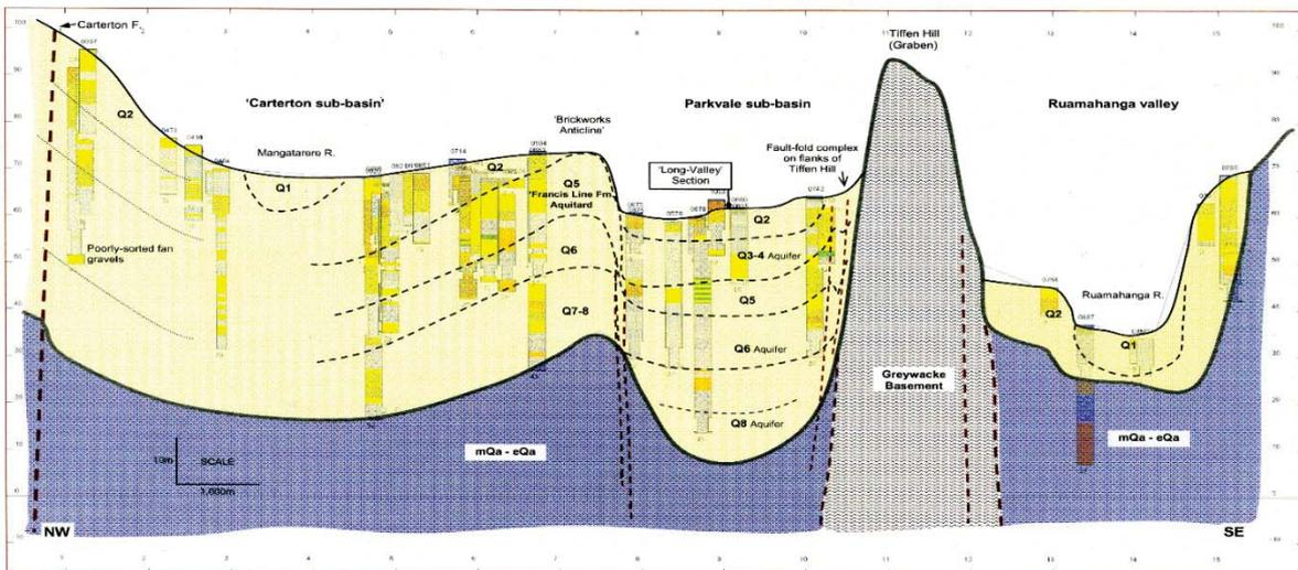
Figure A4.5 Geological cross section 3 (Parkvale - Carterton sub basins). Vertical divisions = 10 m / horizontal = 1 km.
