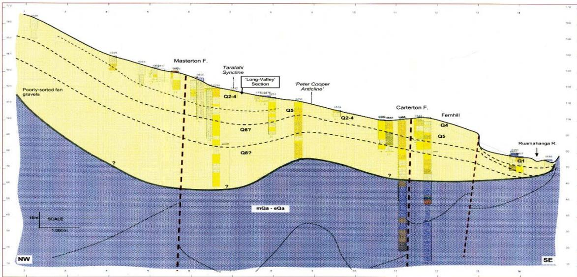
Figure A4.4 Geological cross section 2 (Waingawa fan). Vertical divisions = 10 m / horizontal = 1 km.
