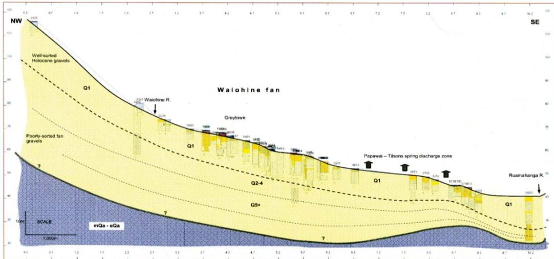
Figure A4.6 Geological cross section 4 (Waiohine fan – Greytown). Vertical divisions = 10 m / horizontal = 1 km.
