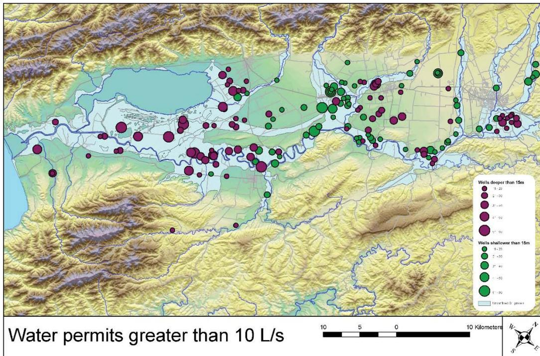
Figure A4.15 Location of groundwater take permits of >10 L/sec in the Wairarapa Valley. Circle size is proportional to take size; purple = wells greater than 15 m depth; green = wells less than 15 m depth.
