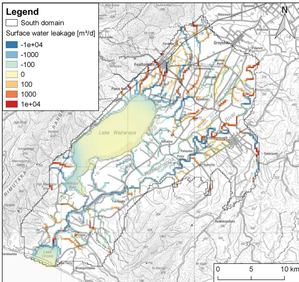
Figure 5.22 Modelled losing and gaining stream reaches in the south model (in this figure negative values indicate a loss from the aquifer or gaining streams, positive is a gain to the aquifer and so losing streams).
