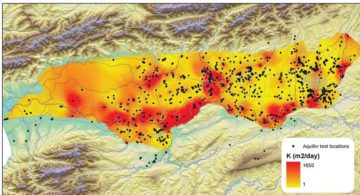
Figure A4.17 Hydraulic conductivity distribution from pumping test analyses in the Wairarapa Valley.
