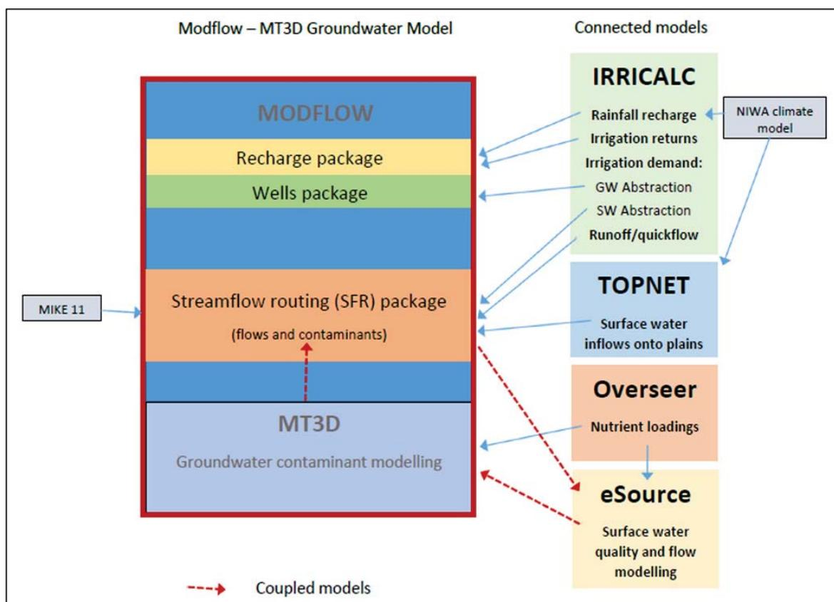
Figure 3.1 Integration of MODFLOW and MT3DMS with other models. Customised transfer scripts were developed to transfer data between models (see Appendix 1)
