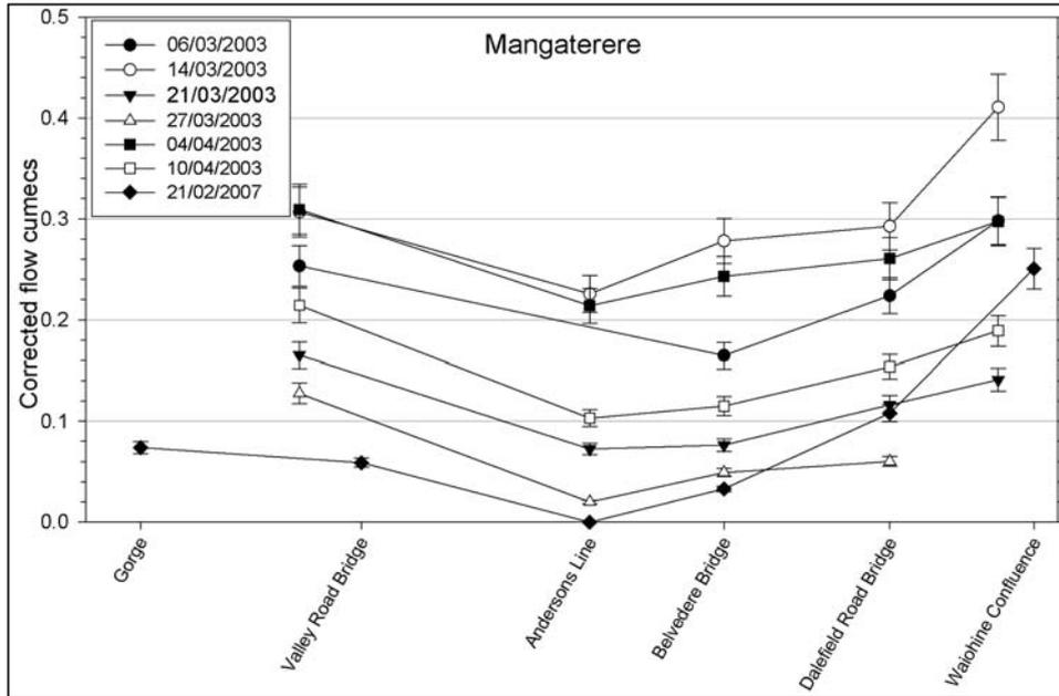
Figure A5.11 Corrected concurrent gauging plots for the Mangatarere Stream.
