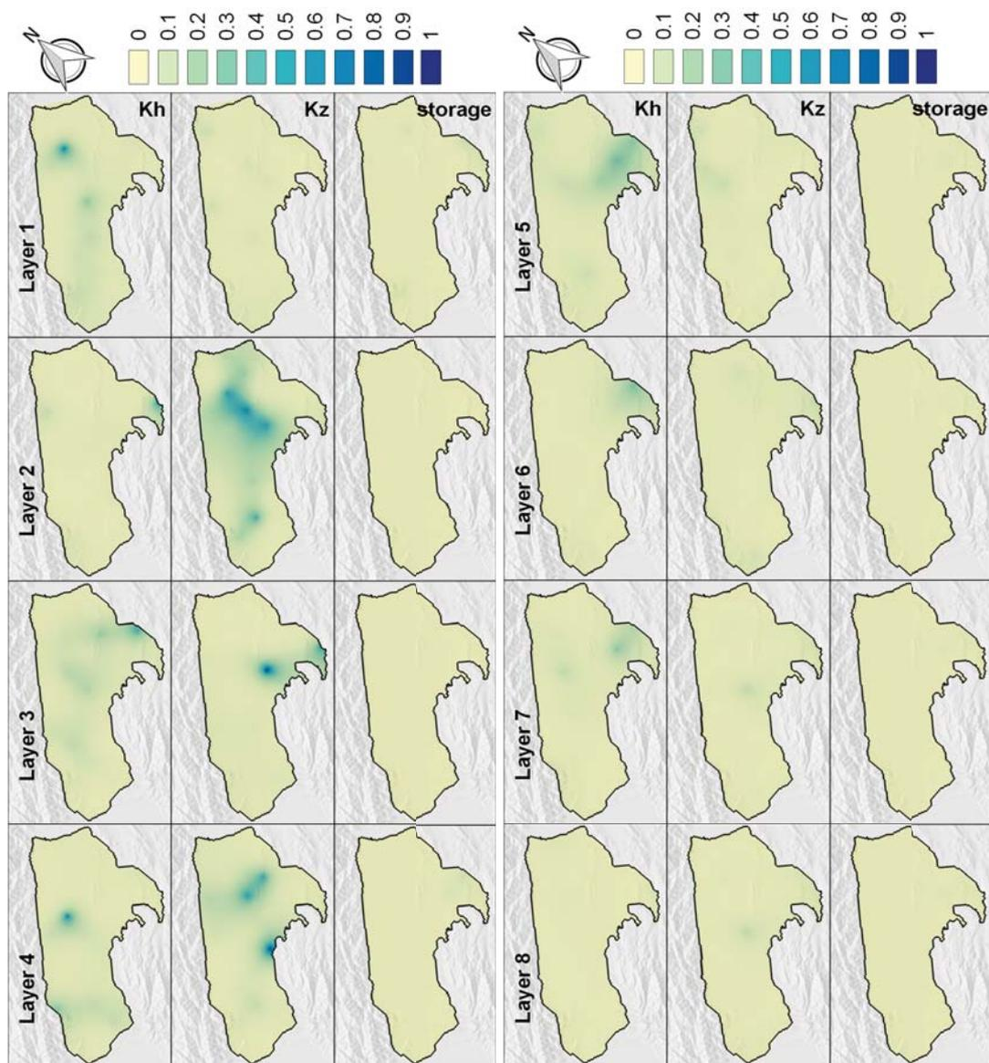
Figure 6.3 Identifiability of hydraulic properties in the south model. Note that storage refers to specific yield in model layer 1 and specific storage in all other model layers.
