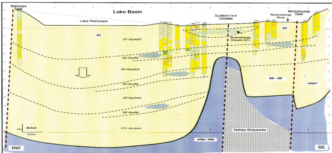
Figure A4.8 Geological cross-section 6 (Lake Wairarapa). Vertical divisions = 10 m / horizontal = 1 km.
