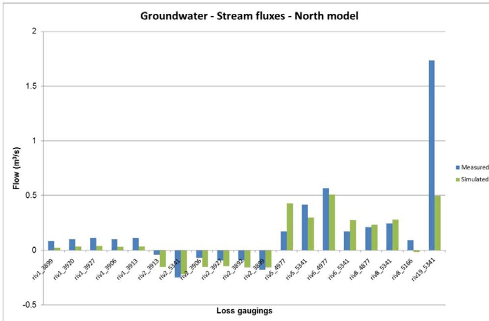
Figure 5.20 Measured and simulated surface water losses and gains for selected river reaches in the north model for various observation times (in this figure negative values indicate a loss to the stream, and positive is a gain to the stream).
