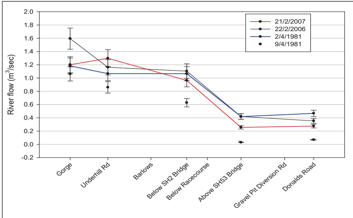
Figure A 5.2 Concurrent flow gauging surveys on the Tauherenikau River.
