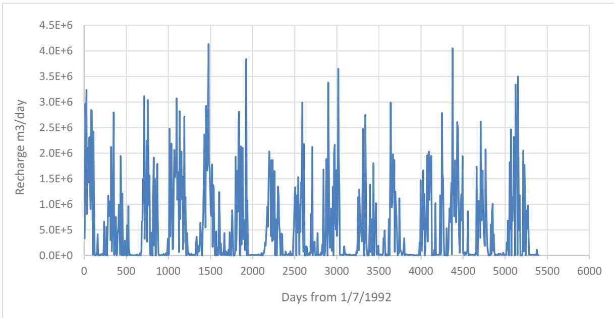
Figure 3.12 Calculated groundwater recharge for the northern model using IRRICALC (Aqualinc, 2016).
