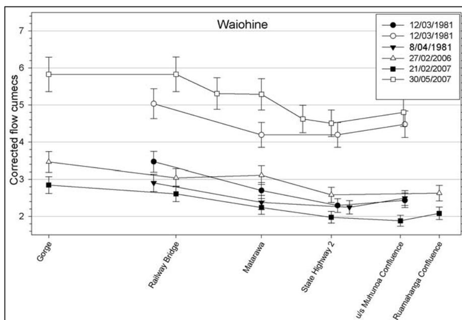
Figure A 5.10 Corrected concurrent gauging plots for the Waiohine River. Where possible, estimated major surface inputs and outputs have been excluded to gain and loss from adjacent groundwater systems.
