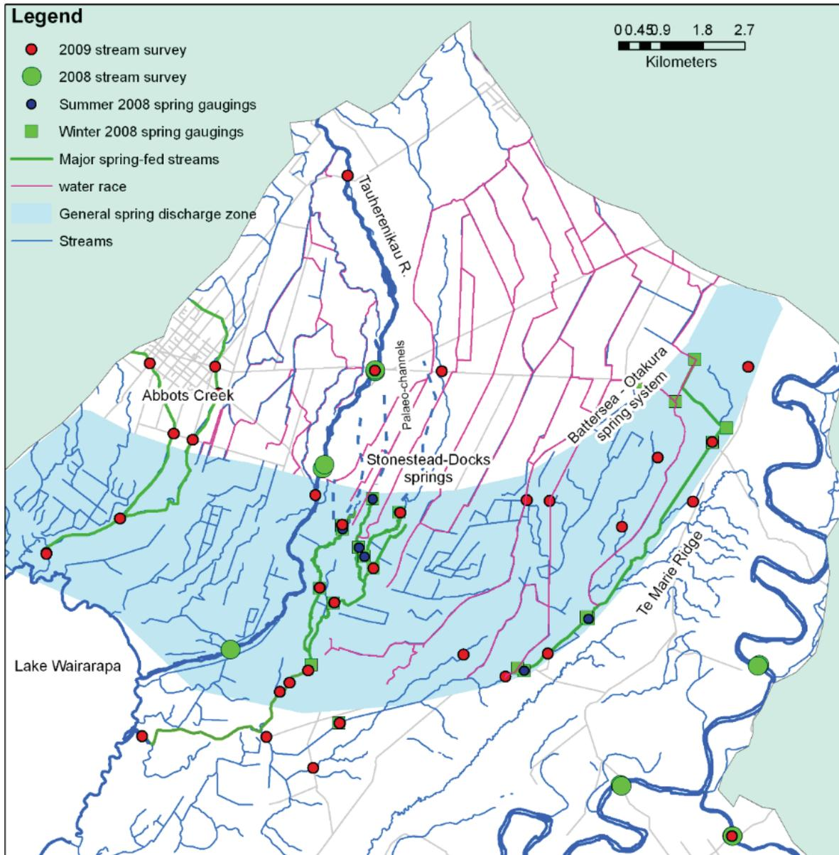
Figure A5.3 Groundwater discharge on the Tauherenikau fan — locations of stream and spring surveys, principal spring-fed streams and general groundwater discharge zone are shown. From Gyopari and McAlister (2010c).
