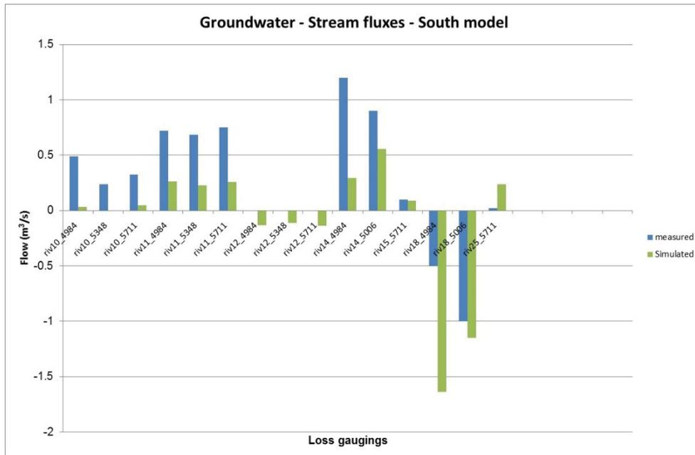
Figure 5.23 Measured and simulated surface water losses and gains for selected river reaches in the south model for various observation times (in this figure negative values indicate a loss to the stream, and positive is a gain to the stream).
