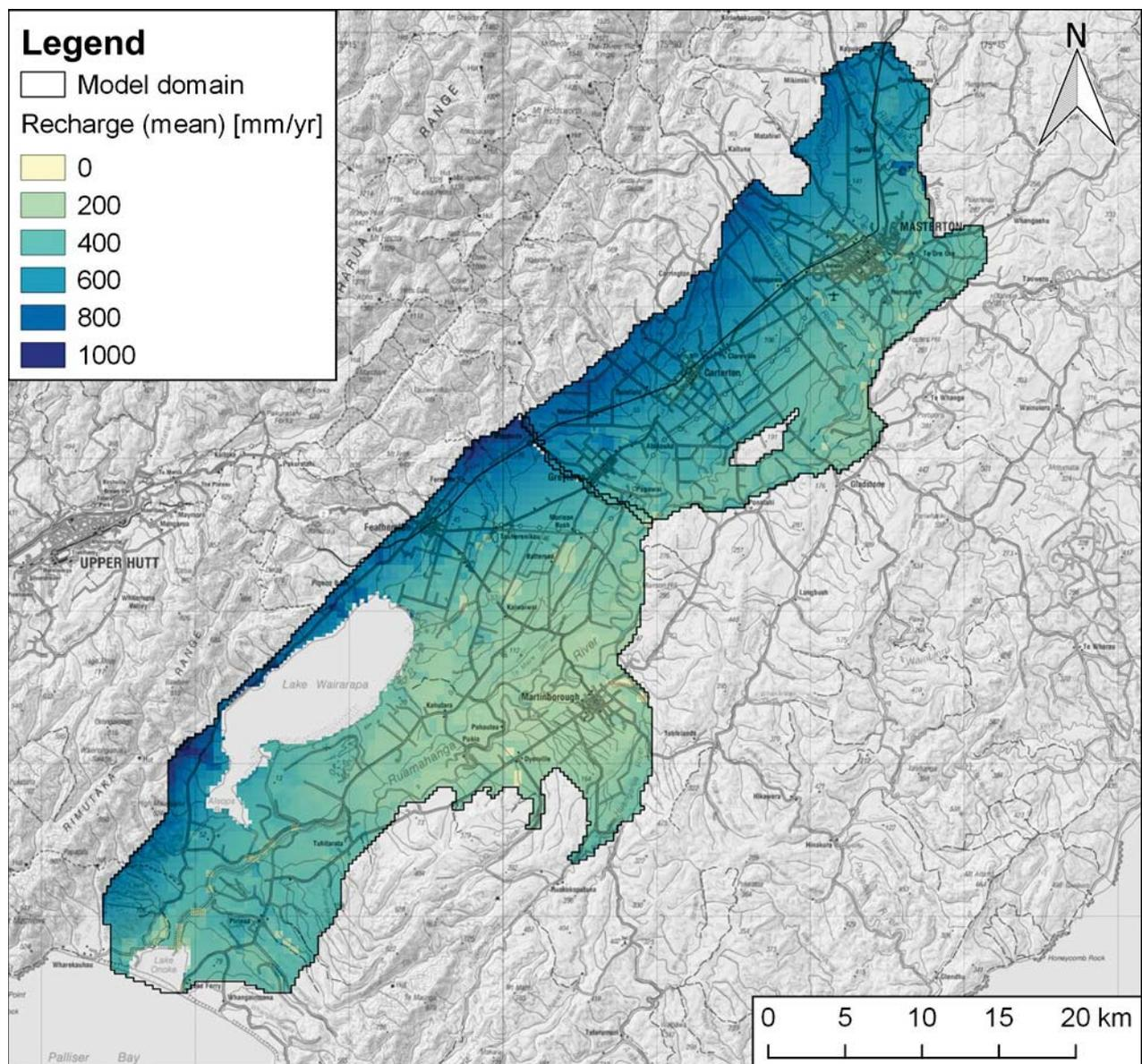
Figure 3.11 Calculated rainfall recharge using IRRICALC in mm/year.
