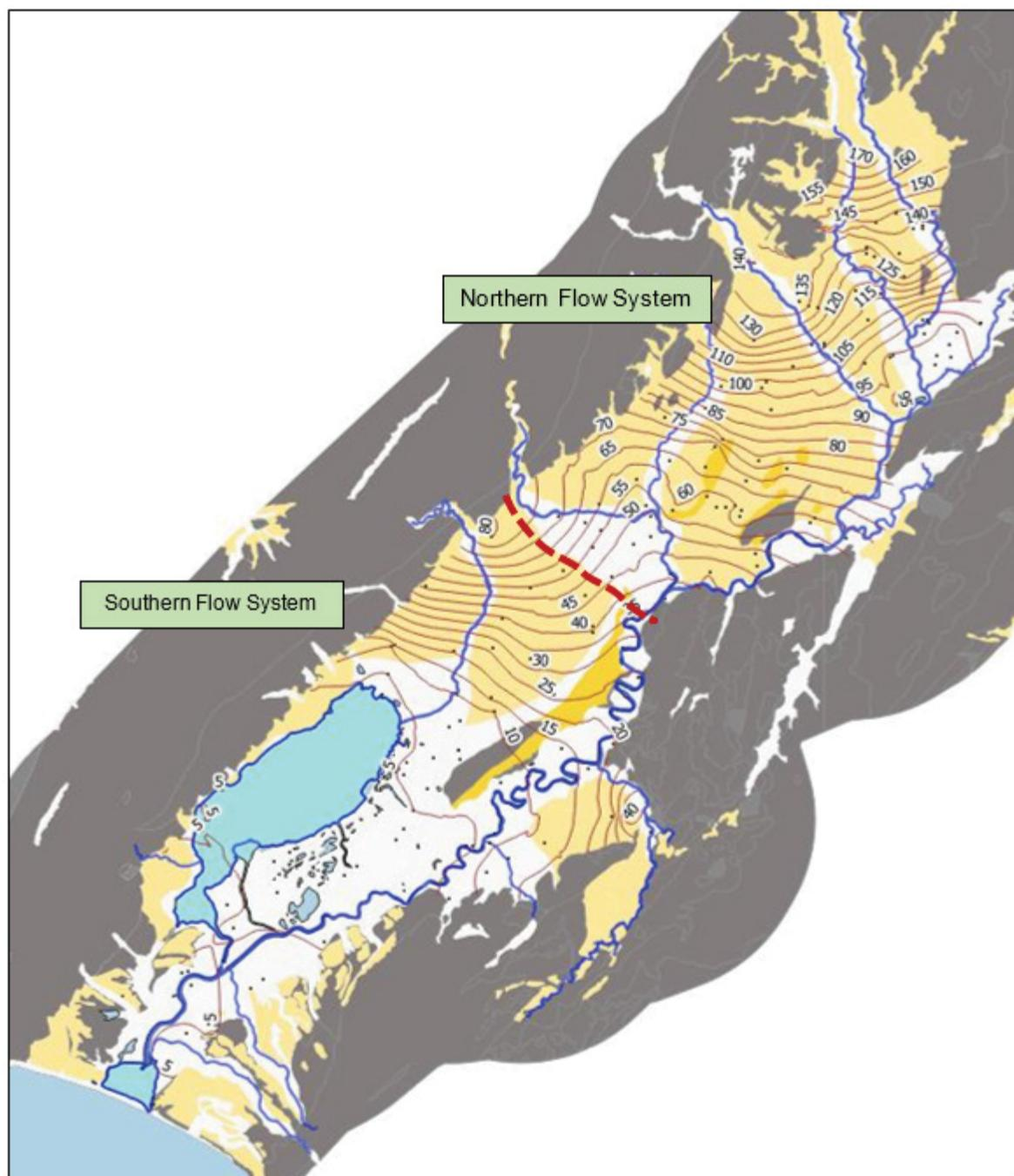
Figure A4.10 Shallow groundwater level contours (March 2007) for the Wairarapa Valley. Data points used to construct the map are also shown. Red dashed line indicates boundary between Northern and Southern Flow Systems along a flow line and geological boundary.
