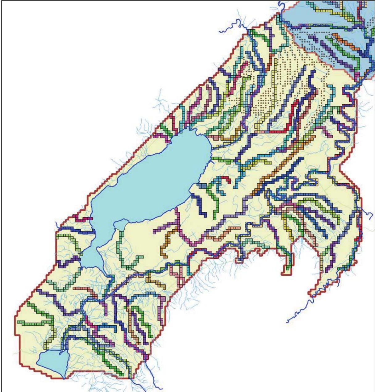
Figure 3.6 SFR1 segments for the southern model for main rivers as well as minor stream and spring-fed drainage systems.
