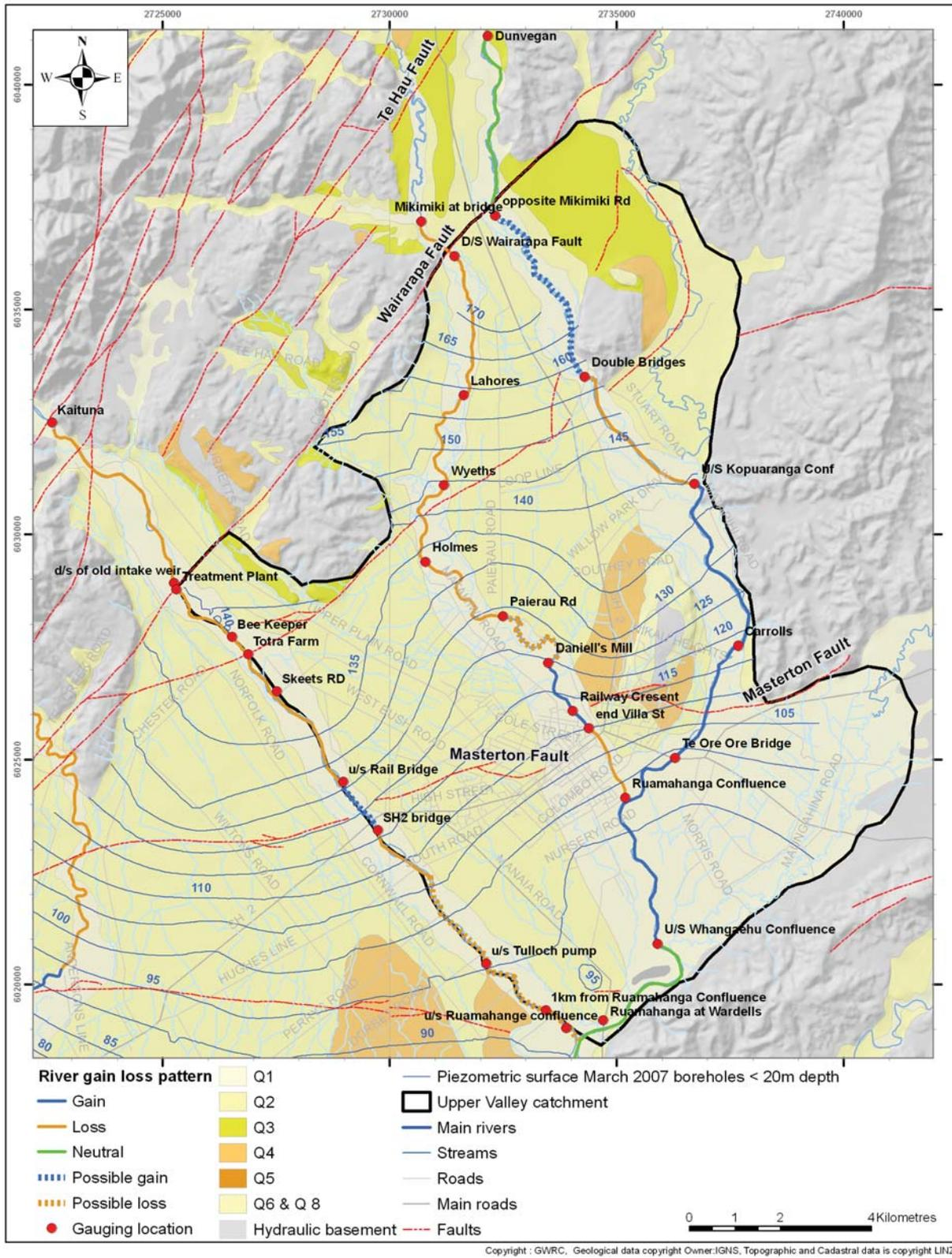
Figure A5.4 Summary of concurrent gauging data showing recognised river gain-loss patterns for the 'upper valley' catchment area of the Northern Flow System (north of the Waingawa River). Groundwater levels contours for March 2007 also shown (in metres above mean sea level). From Gyopari and McAlister (2010a).
