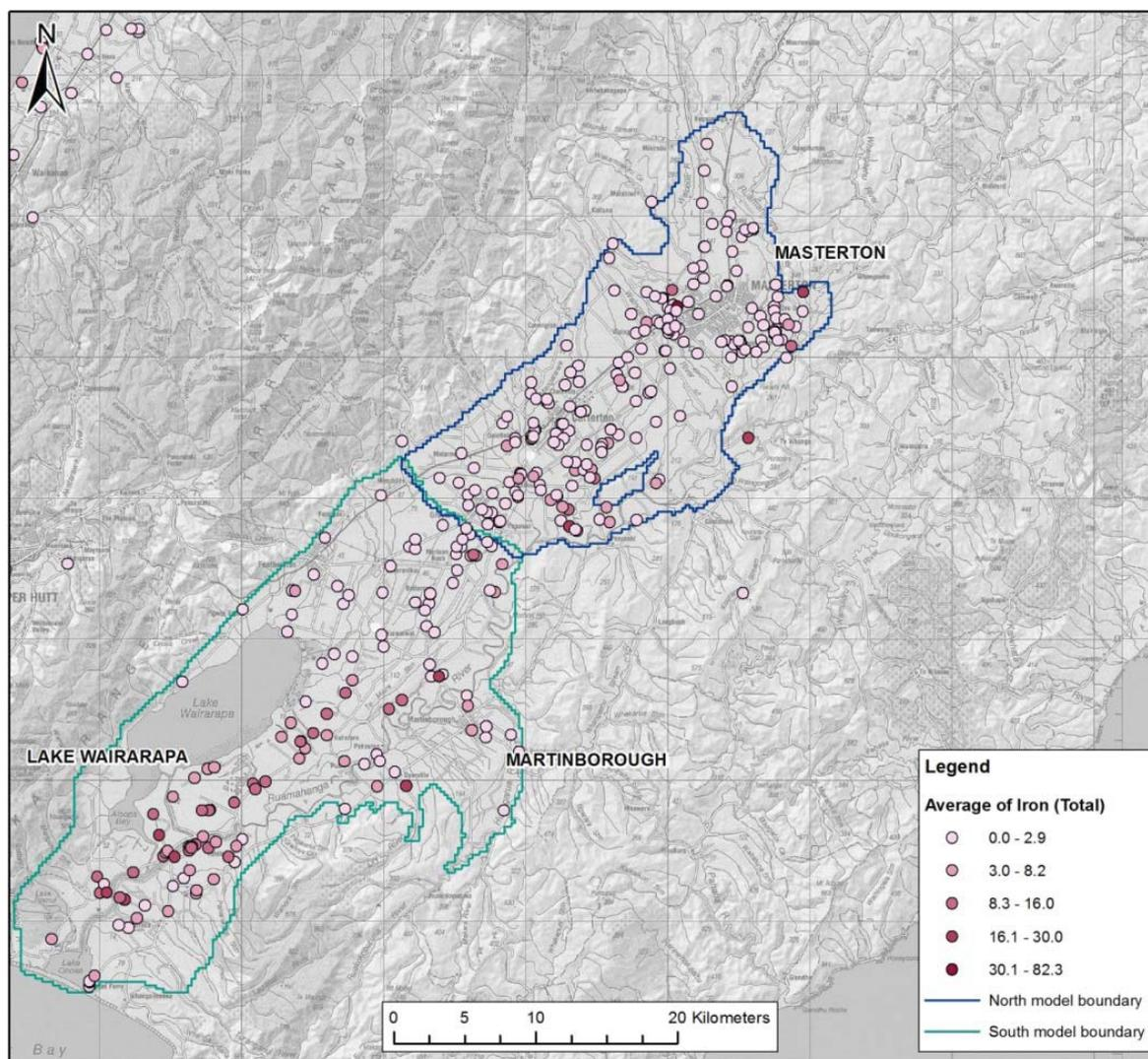
Figure 4.7 Groundwater iron concentration distribution in the Wairarapa Valley.
