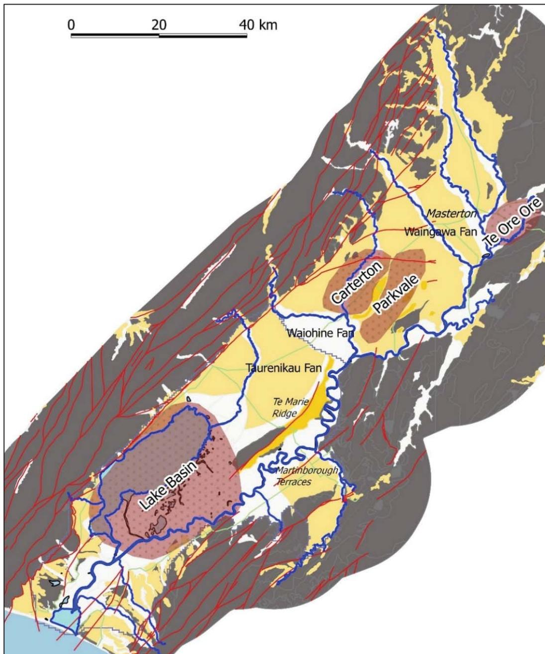
Figure A4.1 Principal hydrogeological features of the Wairarapa Valley. Major faults (red lines) and four sub-basin structures (shaded areas) shown.
