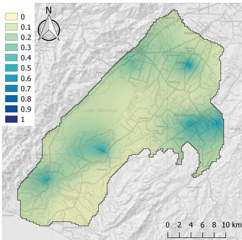
Figure 6.7 Identifiability of recharge multiplier parameters in the south model.
