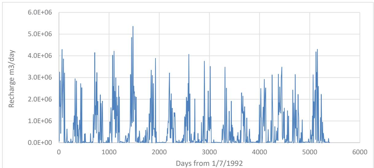
Figure 3.13 Calculated groundwater recharge for the southern model using IRRICALC (Aqualinc, 2016).
