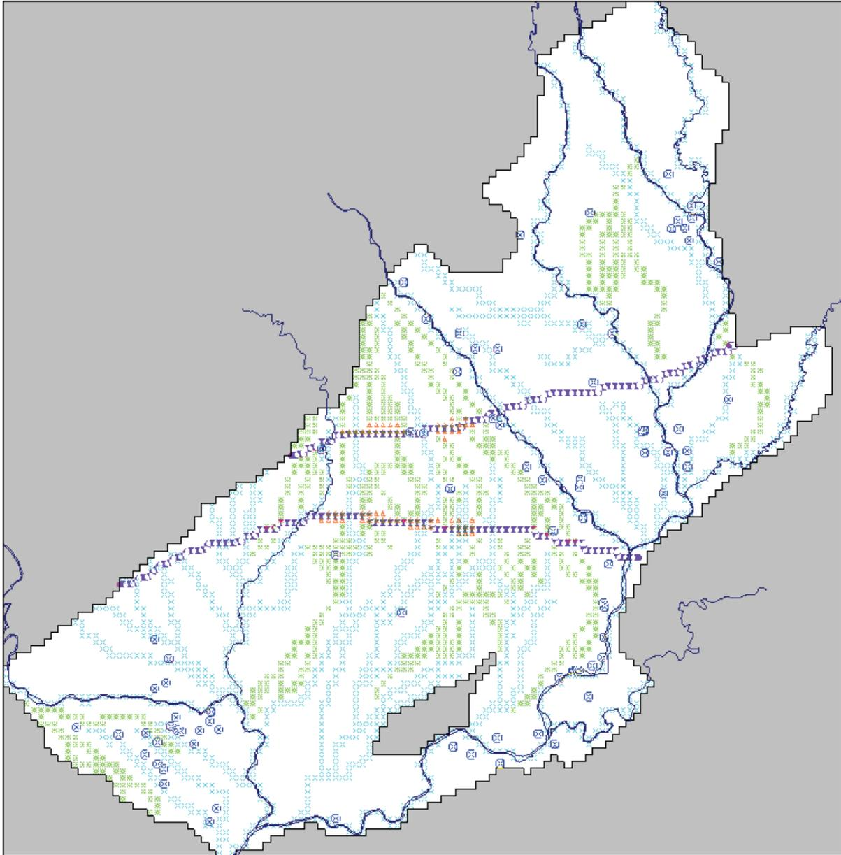
Figure 3.3 Northern model domain showing boundaries, no flow areas (shaded grey) and semi permeable walls representing the Carterton and Masterton regional flow 'barriers' (purple symbols). Other boundary conditions are also shown (SFR = blue symbol; water race injection wells = green symbol; abstraction bores = blue circles; drains/wetlands = orange symbol along faults).
