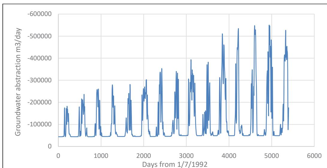
Figure A4.16 Simulated groundwater irrigation demand from groundwater abstraction bores using IRRICALC.
