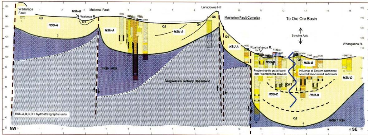
Figure A4.3 Geological cross section 1 (Te Ore Ore / Masterton). Vertical divisions = 10 m / horizontal = 1 km.
