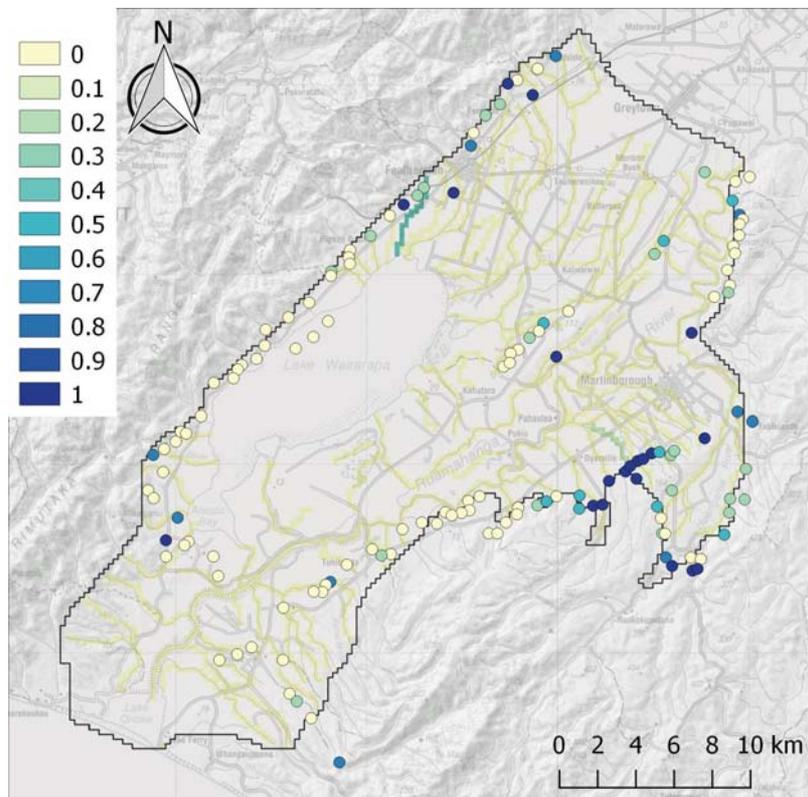
Figure 6.11 Relative parameter uncertainty variance reduction of stream bed conductance parameters and TOPNET model stream multipliers in the south model.
