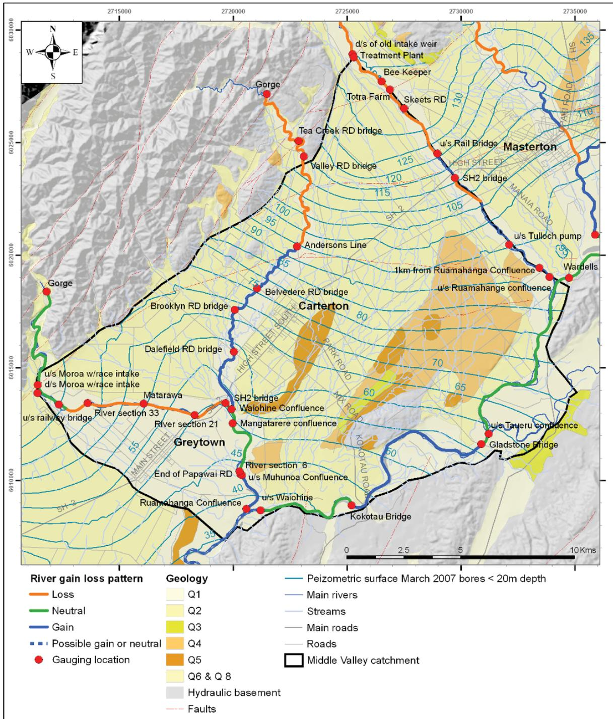
Figure A 5.9 Summary of concurrent gauging data showing recognised river gain-loss patterns for the ‘middle valley catchment’ of the Northern Flow System (south of the Waingawa River). Groundwater levels contours for March 2007 also shown (in metres above mean sea level). From Gyopari and McAlister (2010b)
