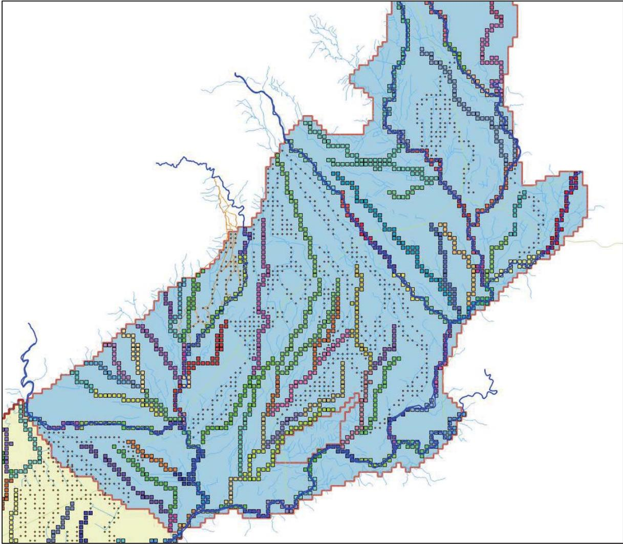
Figure 3.5 SFR1 segments (squares, each segment represented by a different colour) for the northern model for main rivers as well as minor stream and spring-fed drainage systems. Small dots show locations of water race injection wells
