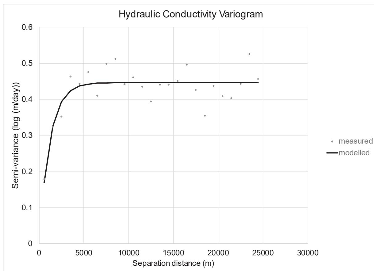
Figure 6.1 Semi-variogram for hydraulic conductivity values (log transformed) in the Ruamāhanga model.
