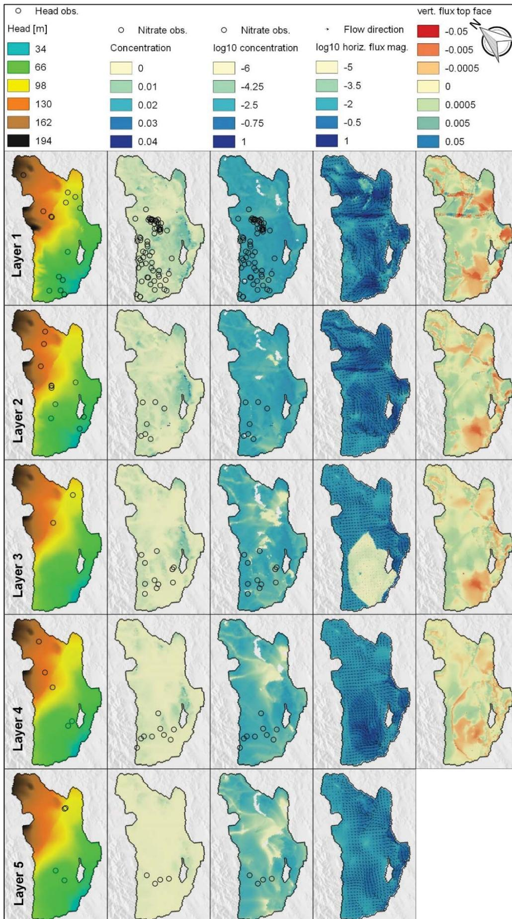
Figure 5.6 Calibrated piezometric, concentration and flux model outputs from the north model calibration.
