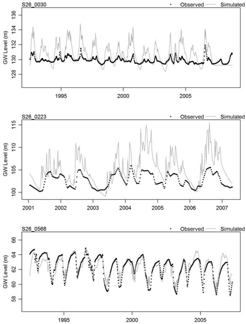
Figure 5.11 Selected modelled and measured groundwater levels in the north model for wells S26/0223, S26/05658 and S26/0030 (refer to Appendix A8 for a complete set of monitoring well modelled-measured groundwater level plots).
