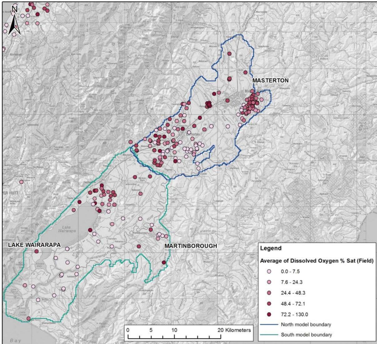
Figure 4.5 Groundwater dissolved oxygen concentration distribution in the Wairarapa Valley.
