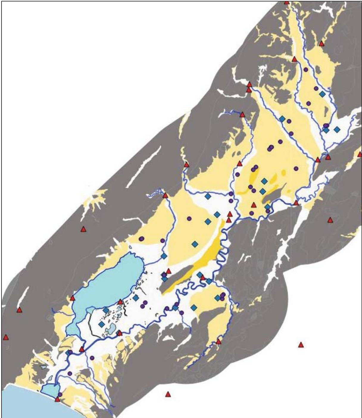
Figure A4.9 Locations of groundwater level monitoring sites (manual – circles; automatic – diamonds) and surface water gauge location (red triangles).
