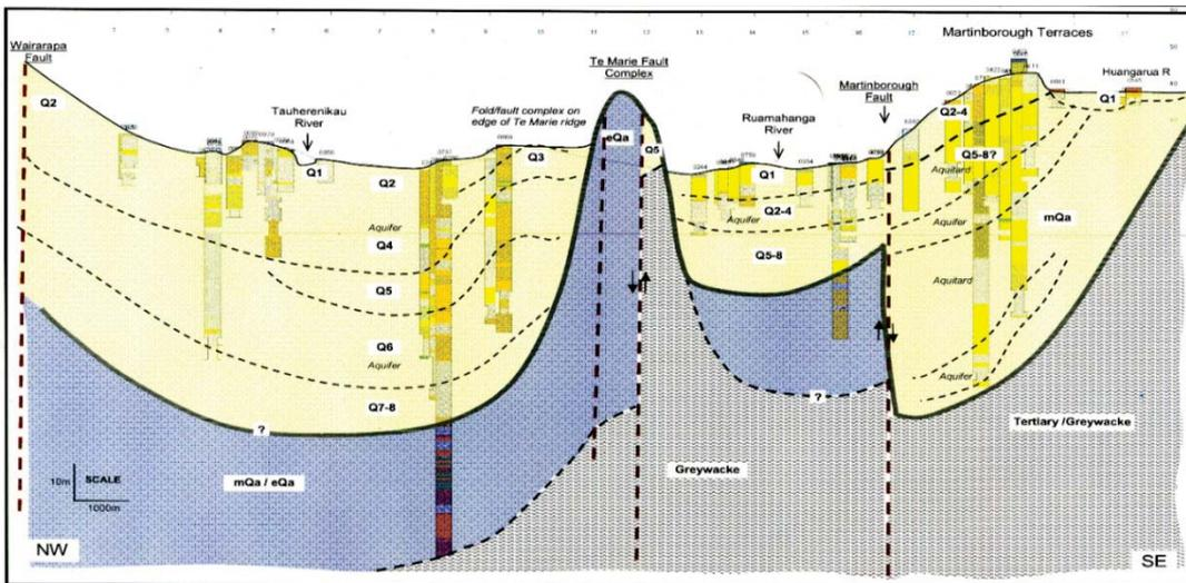
Figure A4.7 Geological cross section 5 (Tauherenikau fan–Te Marie Ridge–Huangarua). Vertical divisions = 10 m / horizontal = 1 km.
