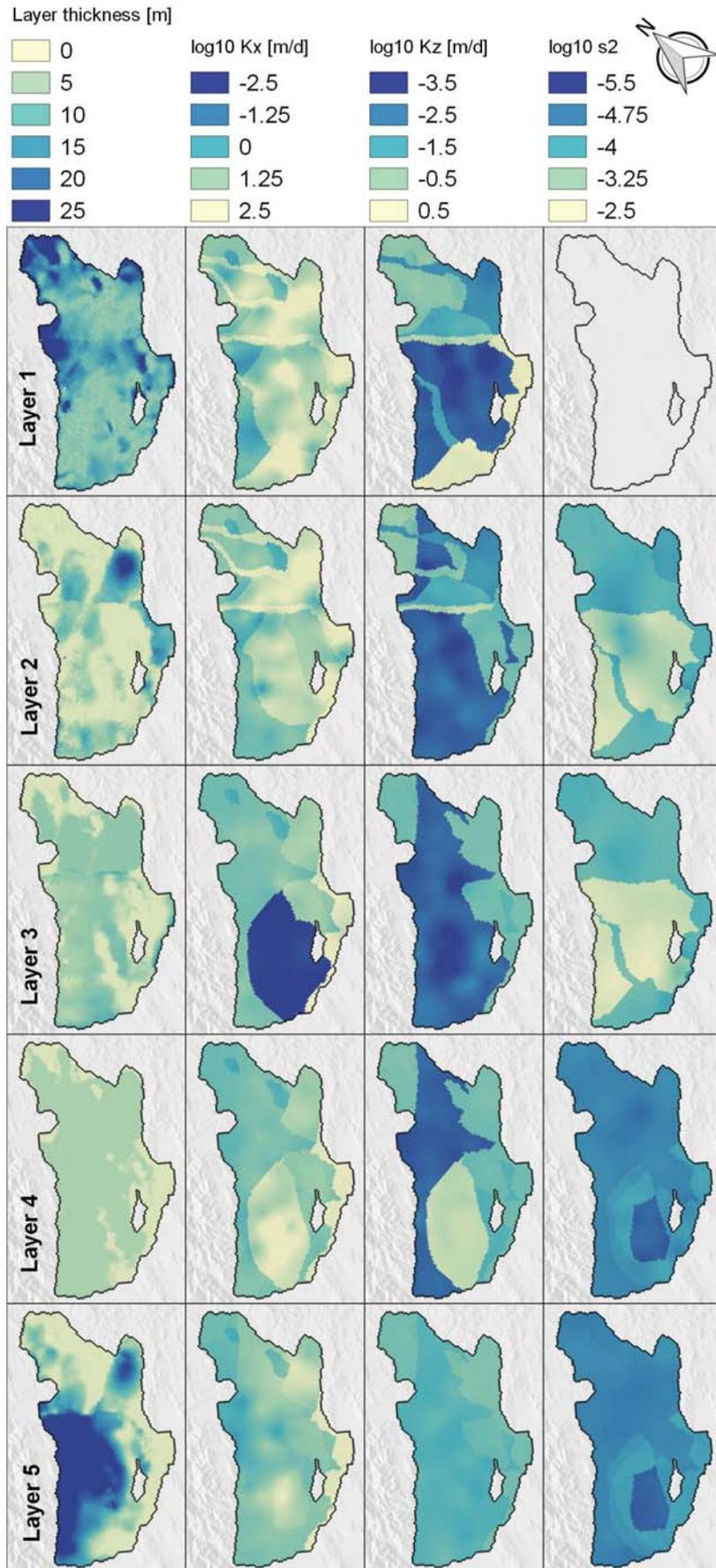
Figure 5.2 Calibrated hydraulic parameter fields from the north model calibration.
