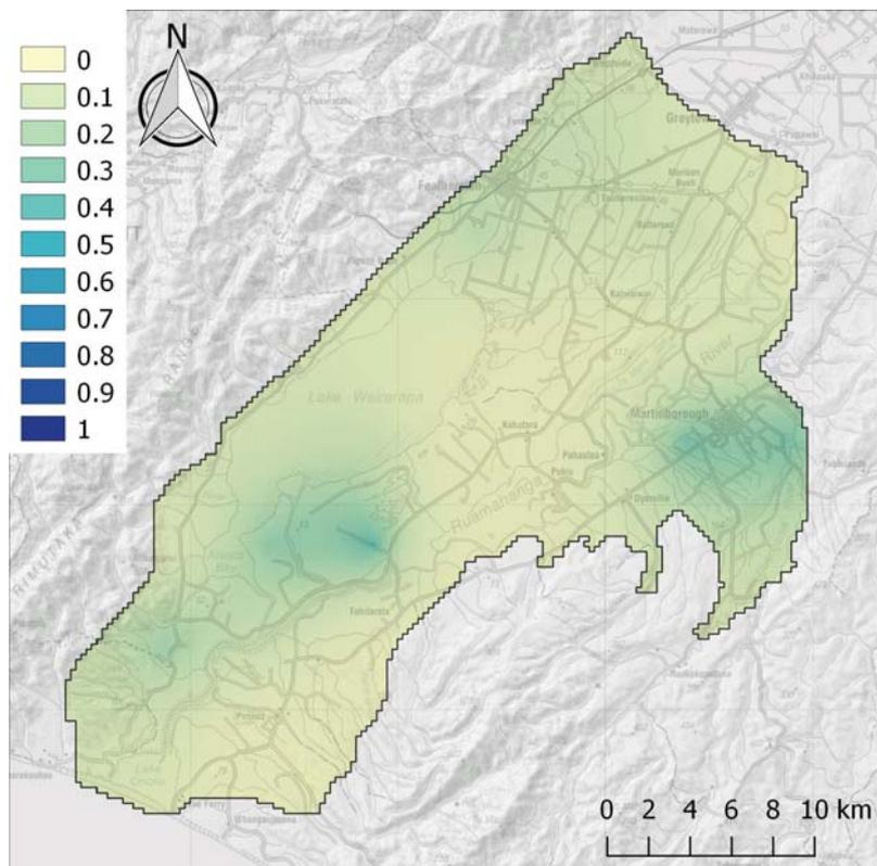
Figure 6.13 Relative parameter uncertainty variance reduction of recharge multiplier in the north model.
