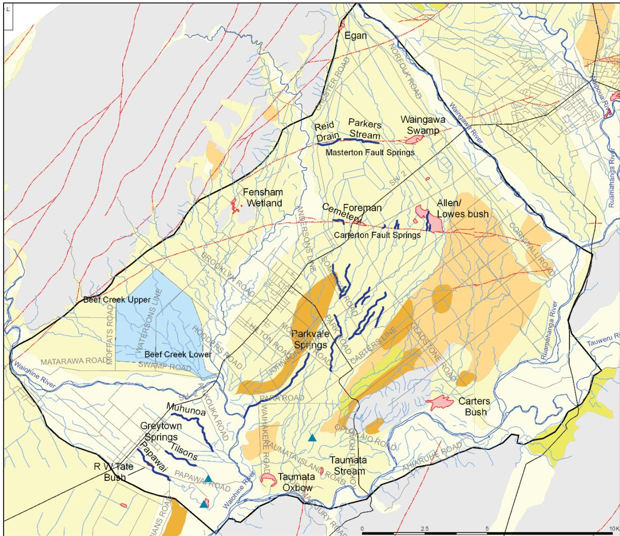
Figure A5.13 Main spring and wetland systems and water races in the middle valley catchment of the Northern Flow System. Heavy blue lines — spring-fed streams; shaded light blue area — widespread spring discharge (Beef Creek system), shaded red area spring-fed wetlands (source: Gyopari and McAlister 2010b)
