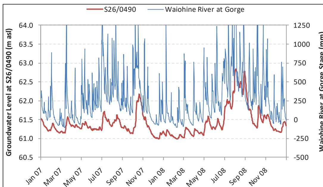
Figure A4.11 Temporal variations in groundwater levels in a shallow bore in the Greytown area (S26/0490) and Waiohine River stage.
