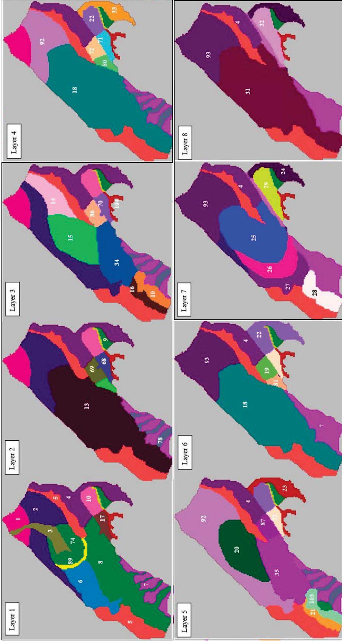
Figure 3.9 Southern model — initial hydraulic conductivity zones.
