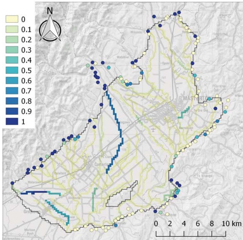
Figure 6.10 Relative parameter uncertainty variance reduction of stream bed conductance parameters and TOPNET model stream multipliers in the north model.
