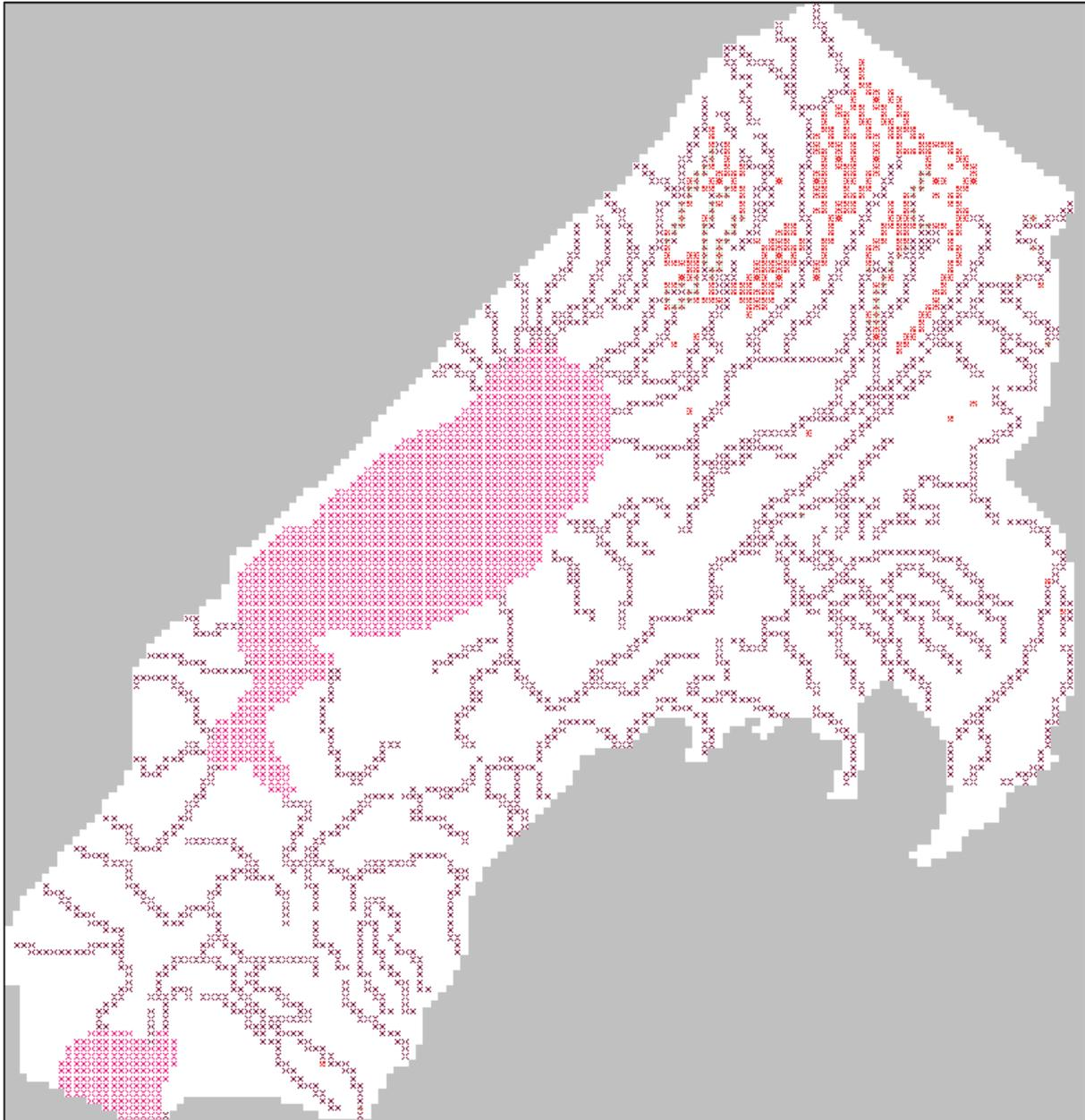
Figure 3.4 Southern model domain showing boundaries, no flow areas (shaded grey). Boundary conditions shown are SFR (purple cross symbol), lake (pink symbol) and water race injection wells (red symbol).
