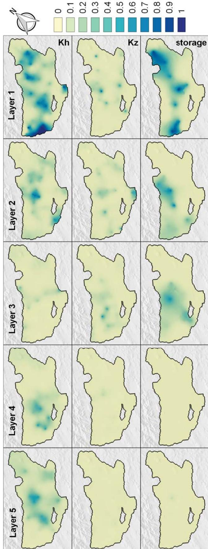
Figure 6.2 Identifiability of hydraulic properties in the north model. Note that storage refers to specific yield in model layer 1 and specific storage in all other model layers.
