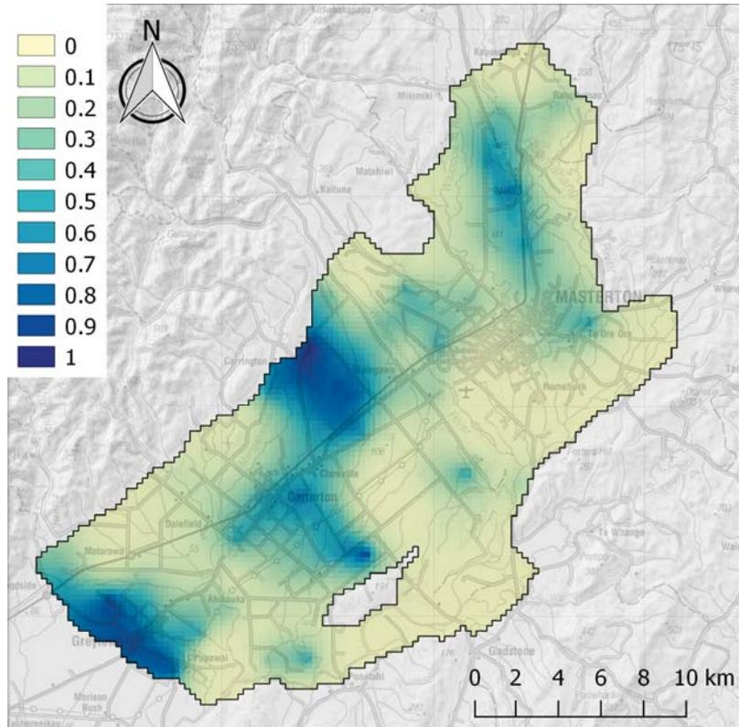
Figure 6.6 Identifiability of recharge multiplier parameters in the north model.
