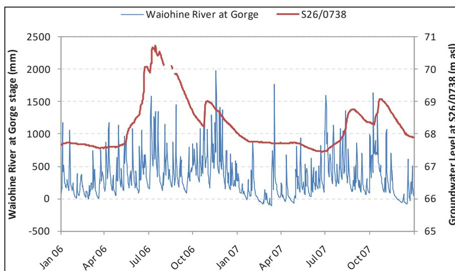
Figure A4.12 Temporal variations in groundwater levels in the unconfined aquifer in the Parkvale area (bore S26/0738) and stage height in the Waiohine River, 2006–07.
