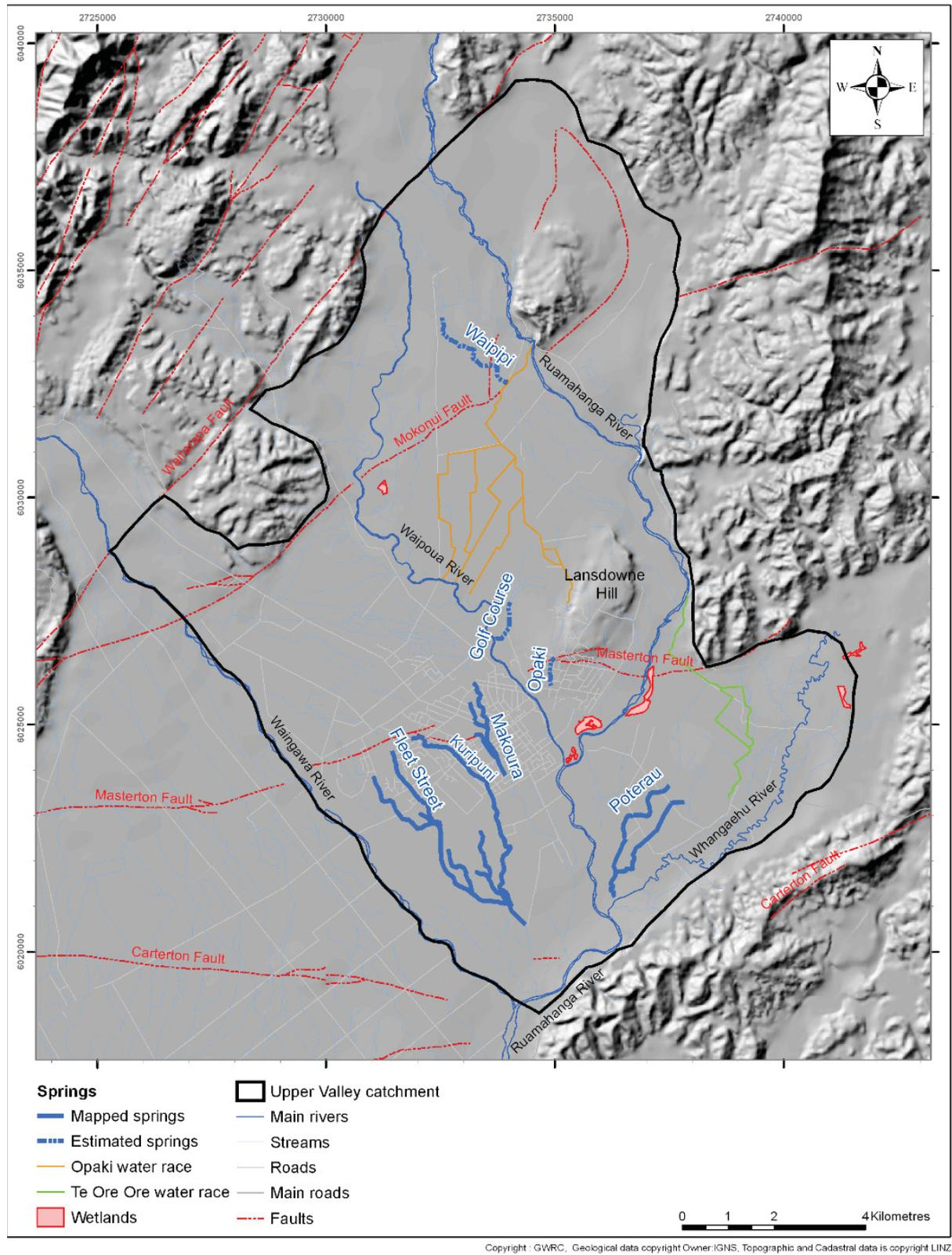
Figure A5.8 Spring discharges, wetlands and water races in the Upper Valley area of the Northern Flow System (Gyopari and McAlister, 2010a).
