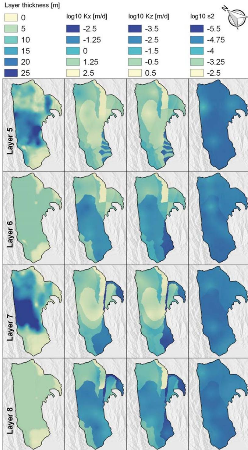
Figure 5.4 Calibrated hydraulic parameter fields from the south model calibration (layers 5–8).
