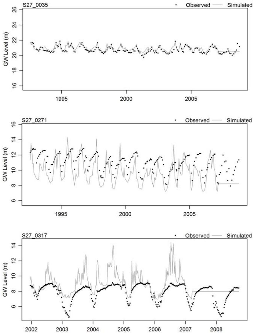
Figure 5.12 Selected modelled and measured groundwater levels in the south model for wells S27/0035, S27/0271 and S27/0317 (refer to Appendix A9 for a complete set of monitoring well modelled-measured groundwater level plots).
