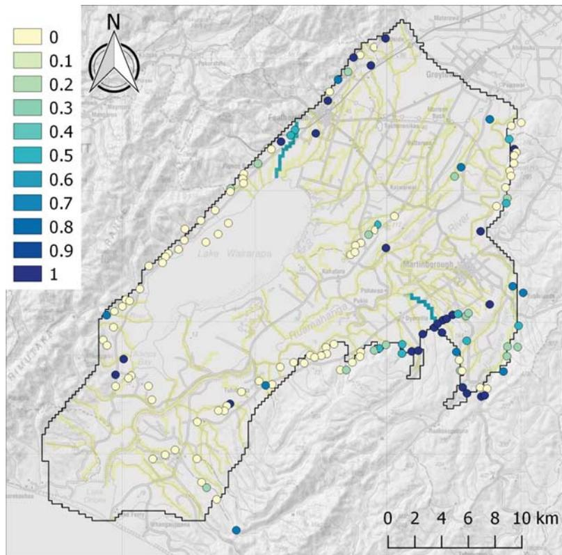
Figure 6.5 Identifiability of stream bed conductance parameters and TOPNET model stream multipliers in the south model.
