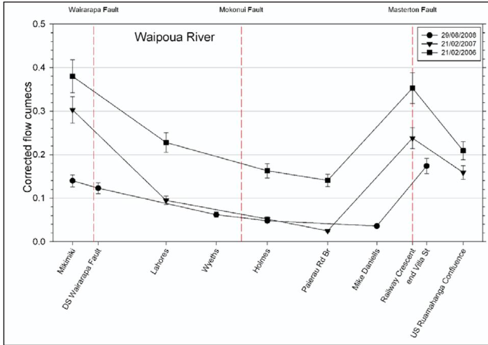
Figure A5.6 Concurrent flow gauging surveys on the Waipoua River.
