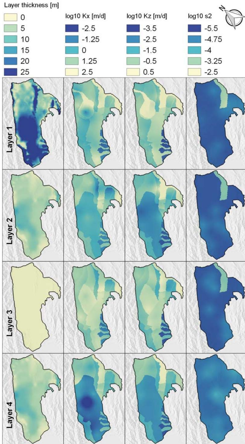
Figure 5.3 Calibrated hydraulic parameter fields from the south model calibration (layers 1–4).
