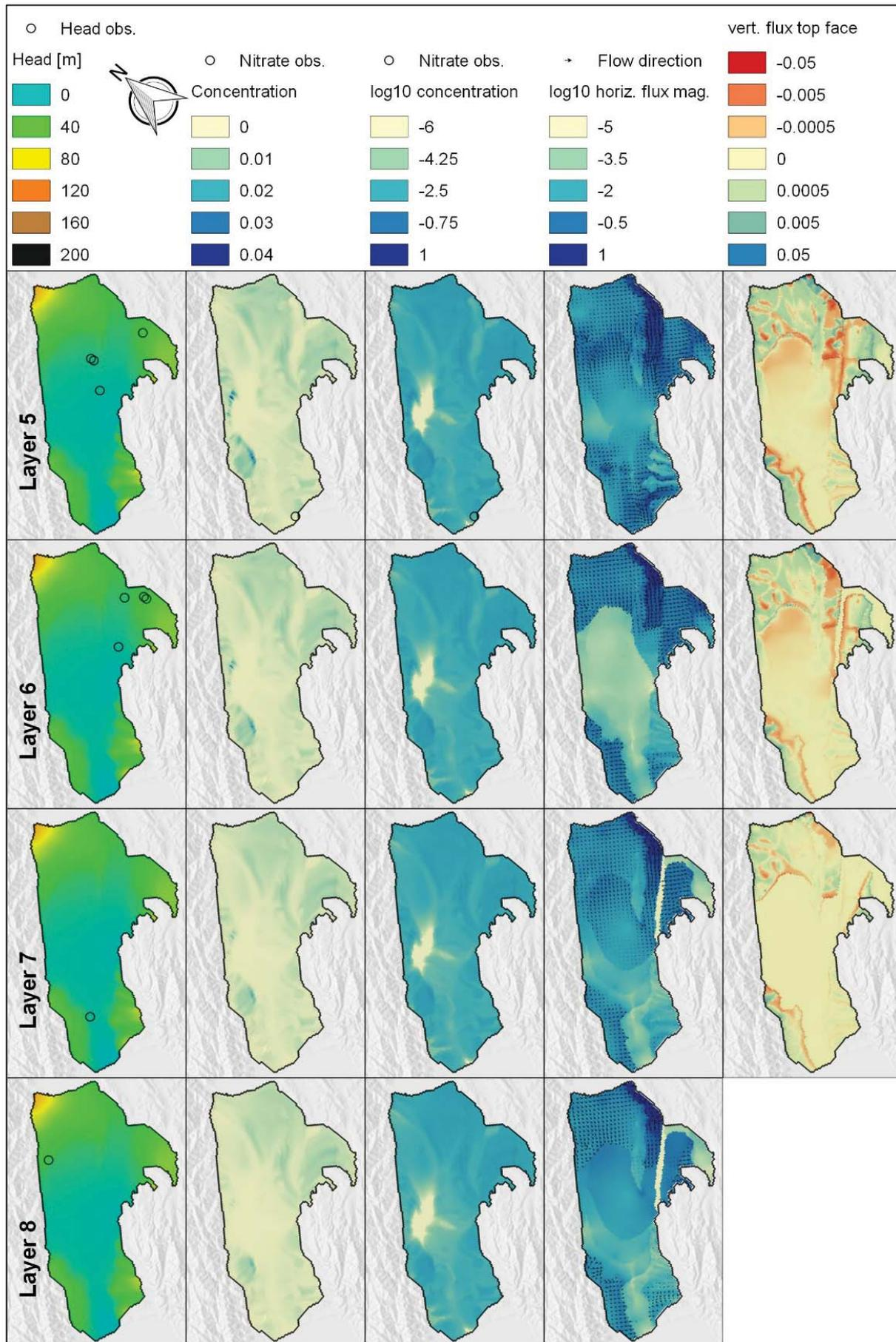
Figure 5.8 Calibrated piezometric, concentration and flux model outputs from the south model calibration (layers 5–8).
