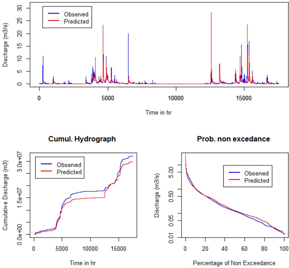
**Figure 4-25: Calibrated hourly hydrograph of Whangaehu at Waihi over the calibration period 2001-2003. Flows are plotted in log scale.**
