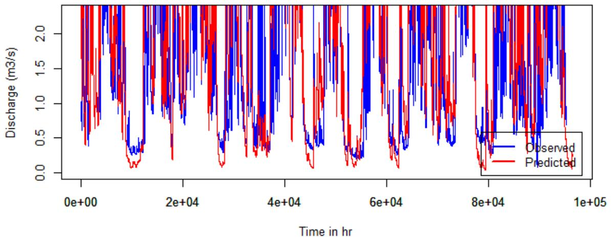
Figure 4-23: Observed and simulated hourly low flow hydrograph (i.e., flow below mean flow) for Kopuaranga at Palmers Bridge over the calibration and validation periods.
