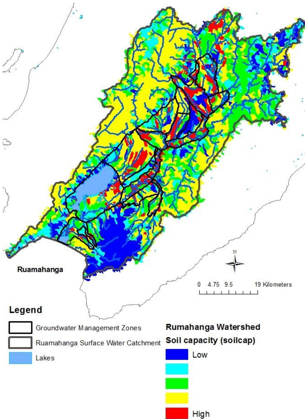
**Figure 3-12: Spatial variation of the soil capacity (soilcap), used as a surrogate of the depth of hydraulically active soil in TopNet. Red represents high values of the parameter, while blue represents low values.**
