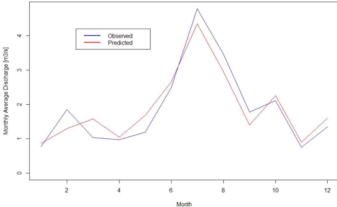
**Figure 4-36: Observed and simulated monthly average flow for Huangarua at Hautotara Branch over the calibration and validation periods.**
