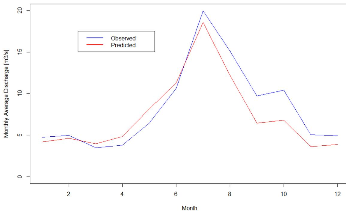
**Figure 4-32: Observed and simulated monthly average flow for Taueru at Te Weraiti over the validation period.**
