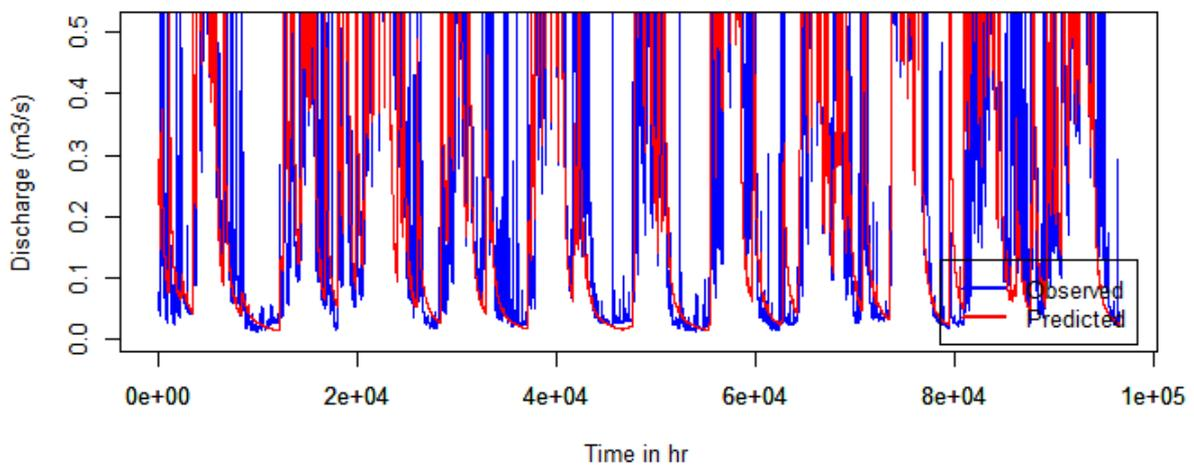
Figure 4-27: Observed and simulated hourly low flow hydrograph (ie flow below mean flow) for Whangaehu at Waihi over the calibration period and validation periods.
