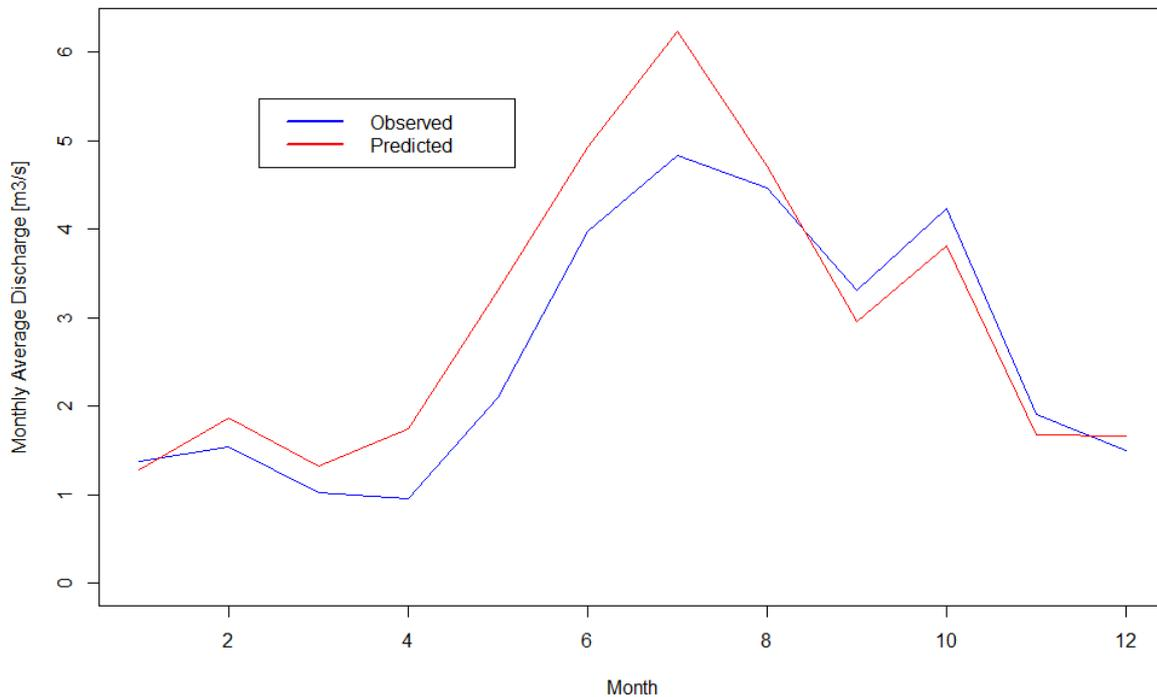
**Figure 4-24: Observed and simulated monthly average flow for Kopuaranga at Palmers Bridge over the validation period.**
