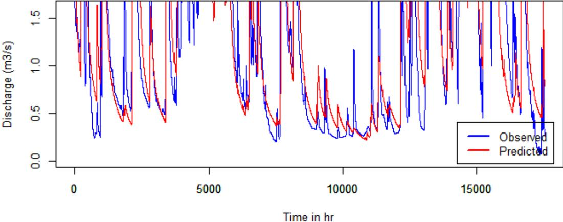
**Figure 4-35: Observed and simulated hourly low flow hydrograph (i.e., flow below mean flow) for Huangarua at Hautotara Branch over the calibration and validation periods.**
