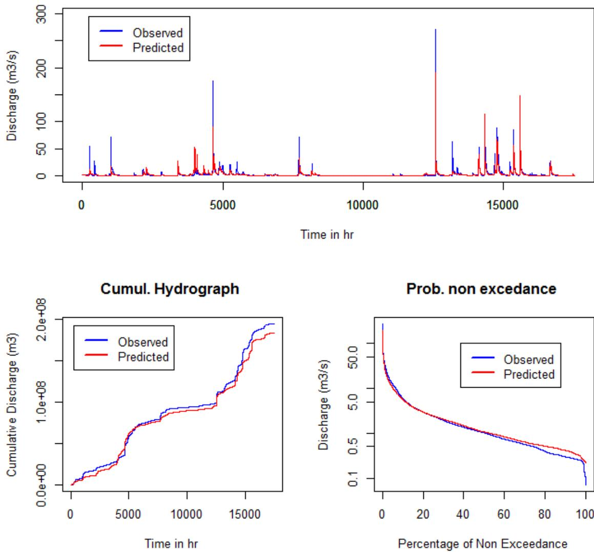
**Figure 4-33: Calibrated hourly hydrograph of Huangarua at Hautotara Branch over the calibration period 2001-2003.**
