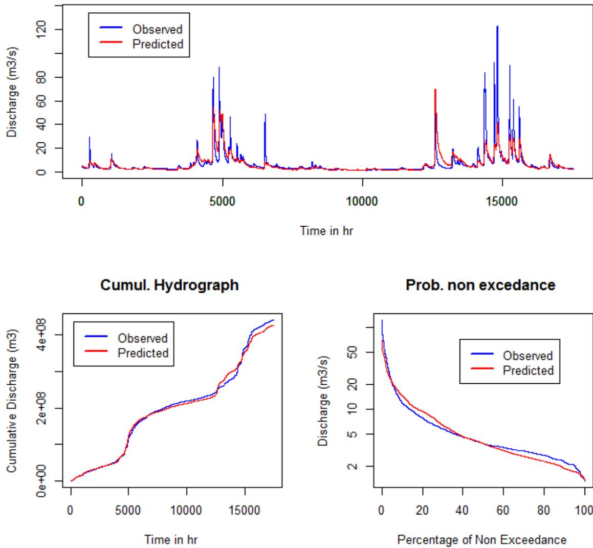
**Figure 4-29: Calibrated hourly hydrograph of Taueru at Te Weraiti over the calibration period 2001-2003.**
