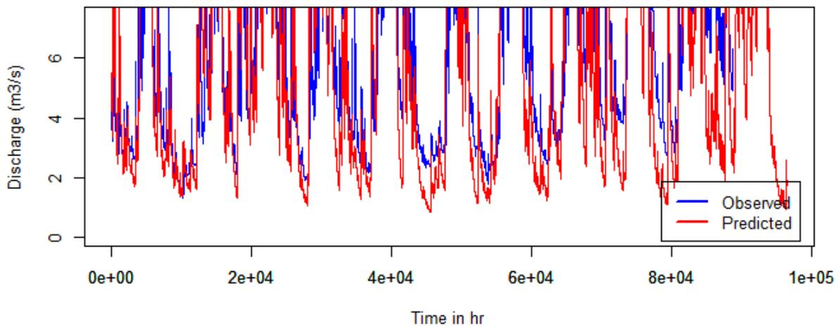
Figure 4-31: Observed and simulated hourly low flow hydrograph (i.e., flow below mean flow) for Taueru at Te Weraiti over the calibration and validation periods.
