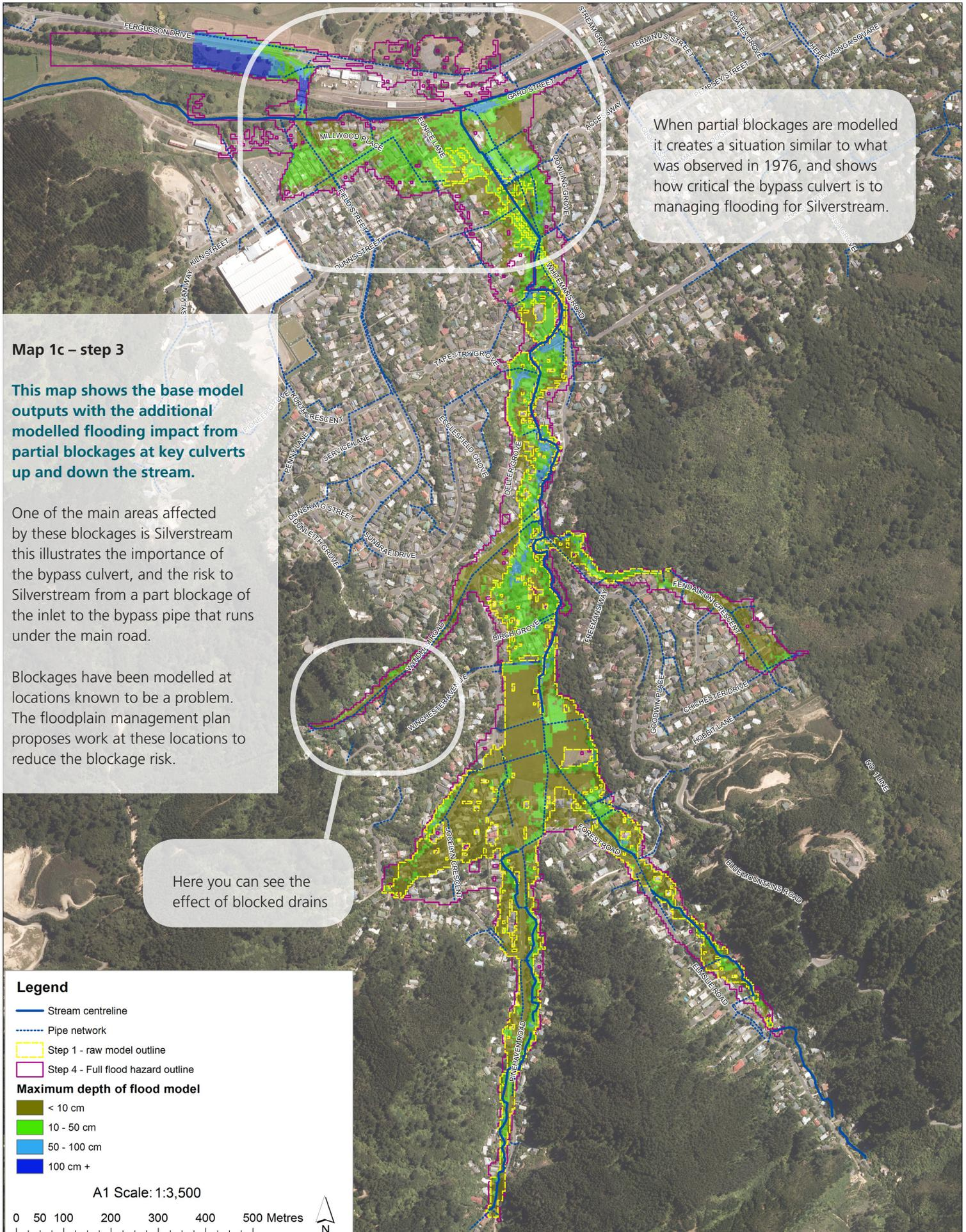
When partial blockages are modelled it creates a situation similar to what was observed in 1976, and shows how critical the bypass culvert is to managing flooding for Silverstream.
