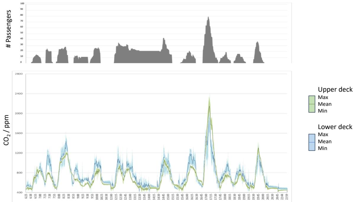
**Figure A-4: CO<sub>2</sub> and number of passengers on 18<sup>th</sup> April 2023 (recirculated air).**
