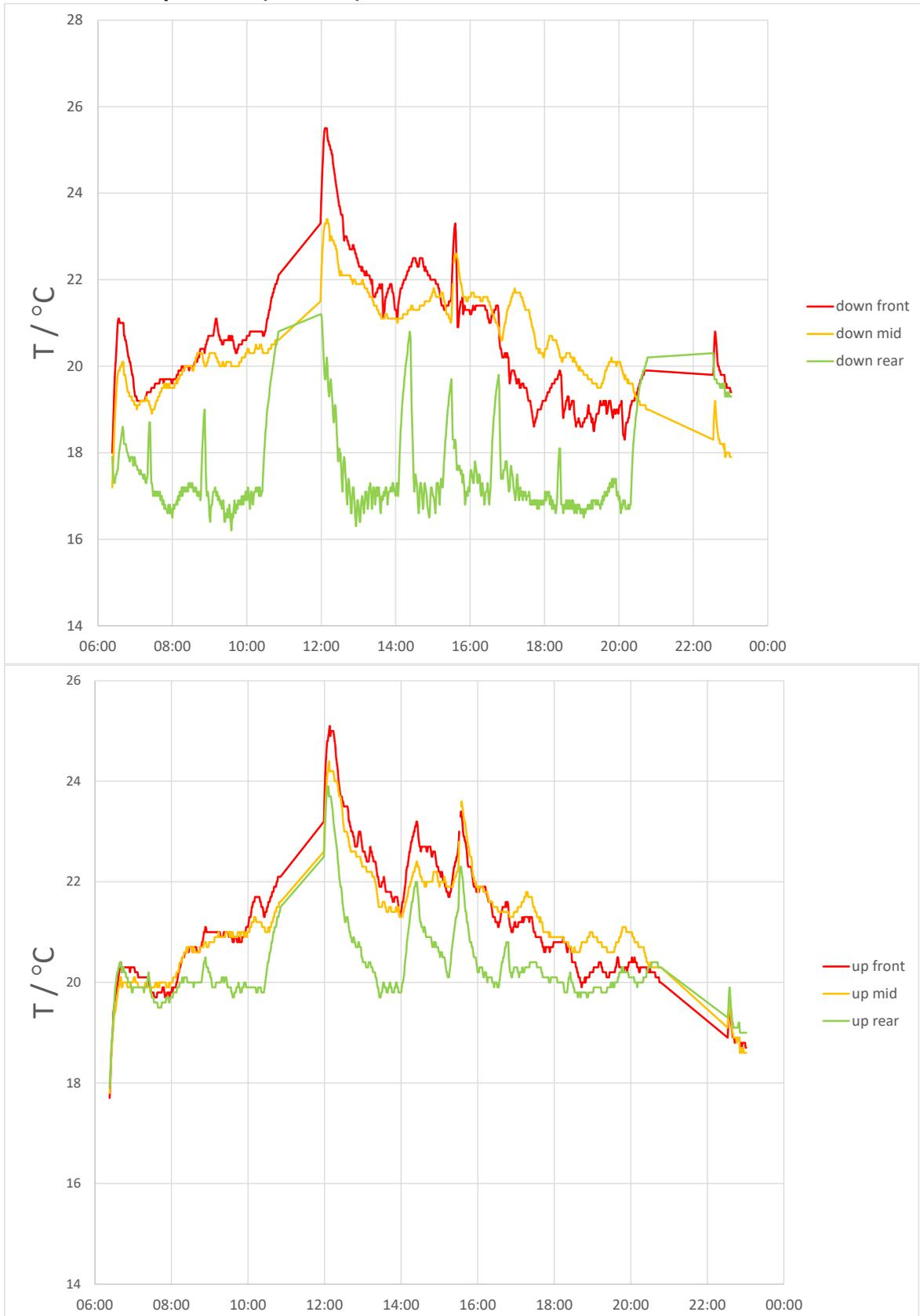
Figure A-14: Temperature at three points each on the lower (left) and upper (right) decks on 18<sup>th</sup> April 2023 (recirculated air).
