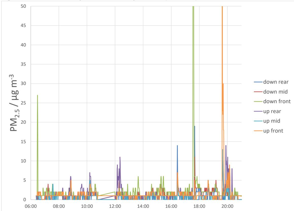
Figure A-9: PM<sub>2.5</sub> at six points on 18<sup>th</sup> April 2023 (recirculated air).
