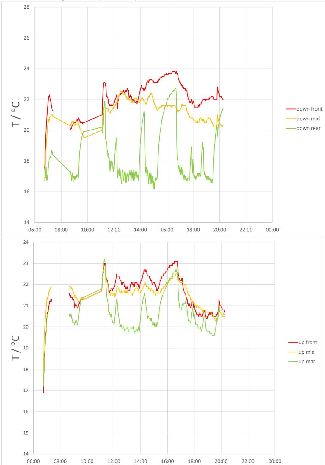
Figure A-13: Temperature at three points each on the lower (left) and upper (right) decks on 13<sup>th</sup> April 2023 (fresh air).
