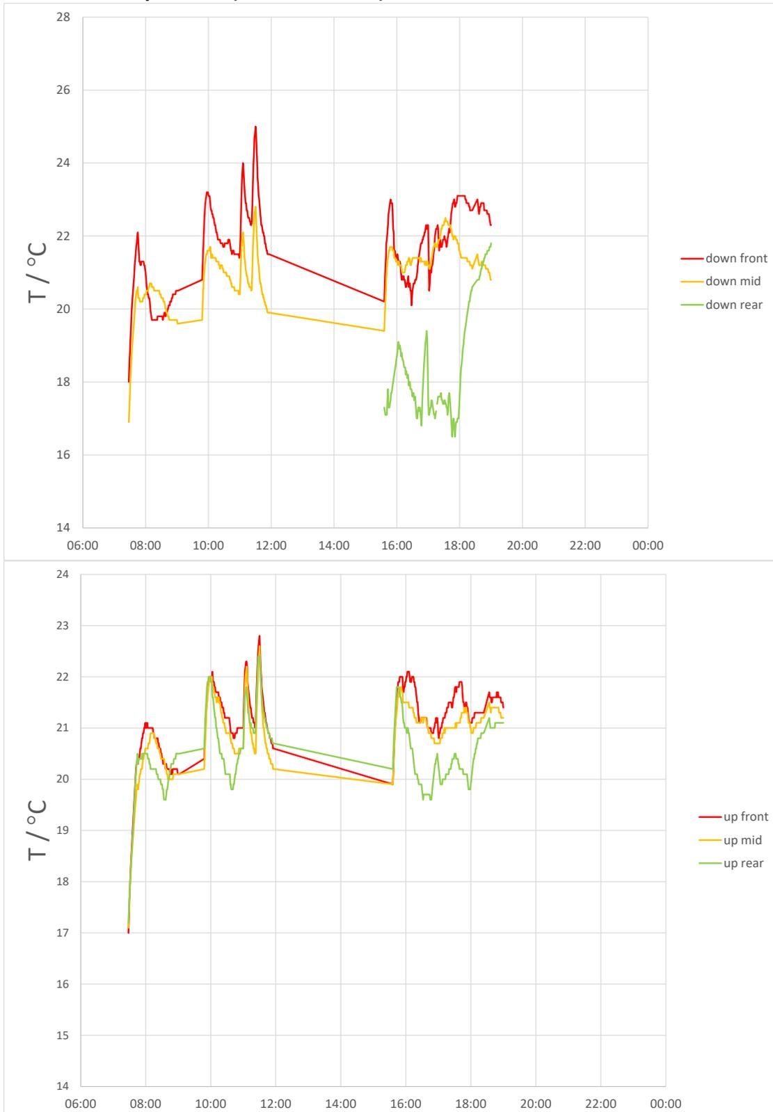
**Figure A-15: Temperature at three points each on the lower (left) and upper (right) decks on 19<sup>th</sup> April 2023 (recirculated air).**
