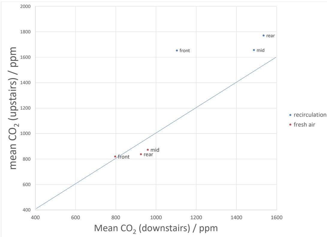
**Figure 2: Comparison of all-study mean CO<sub>2</sub> concentrations on the upper and lower decks as a function of ventilation mode.**
