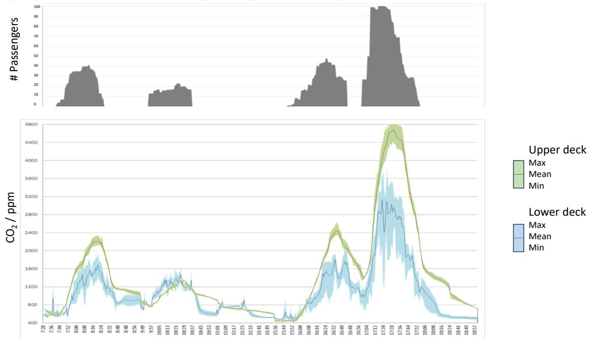
Figure A-5: CO<sub>2</sub> and number of passengers on 19<sup>th</sup> April 2023 (recirculated air).
