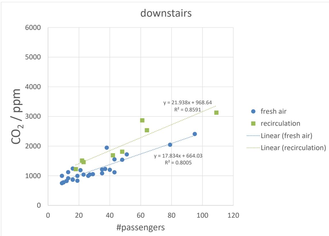
**Figure 4: Relationship between maximum CO<sub>2</sub> concentration on the lower deck and maximum number of passengers for each service run.**
