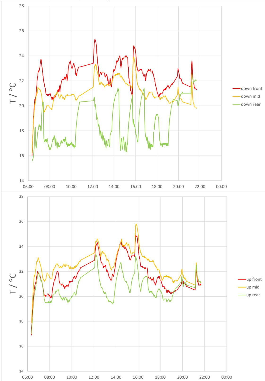
Figure A-12: Temperature at three points each on the lower (left) and upper (right) decks on 12<sup>th</sup> April 2023 (fresh air).
