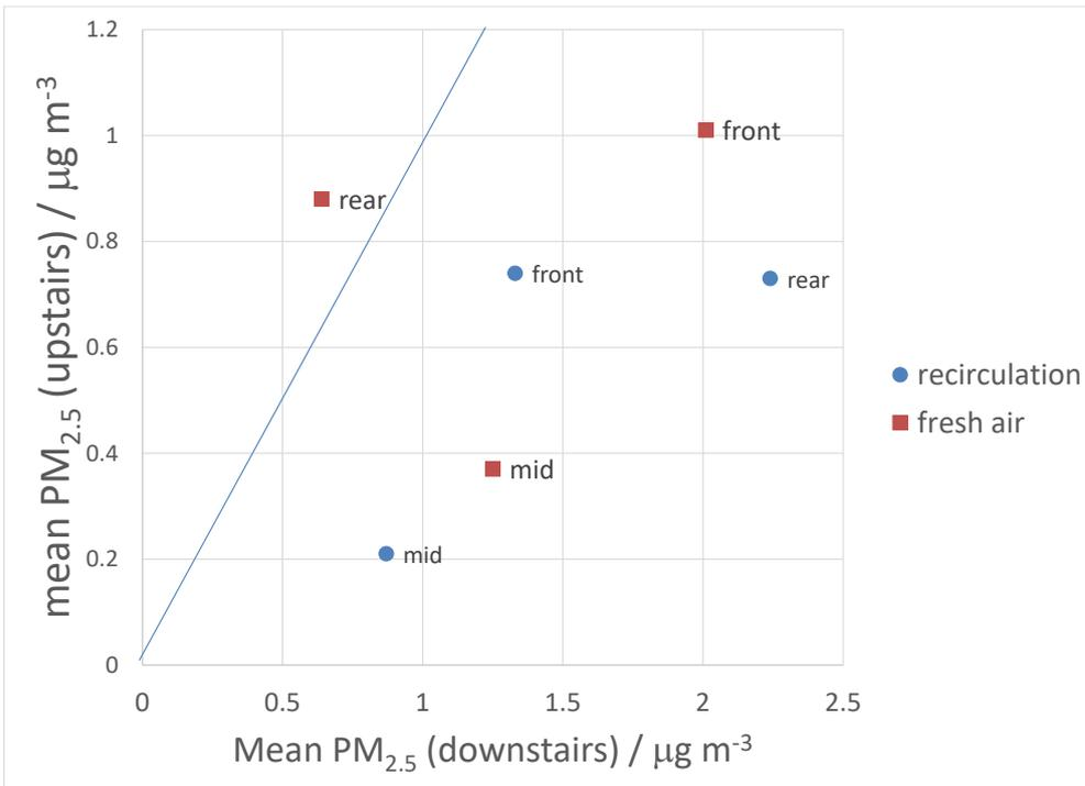
**Figure 7: Comparison of all-study mean PM<sub>2.5</sub> concentrations on the upper and lower deck as a function of ventilation mode.**
