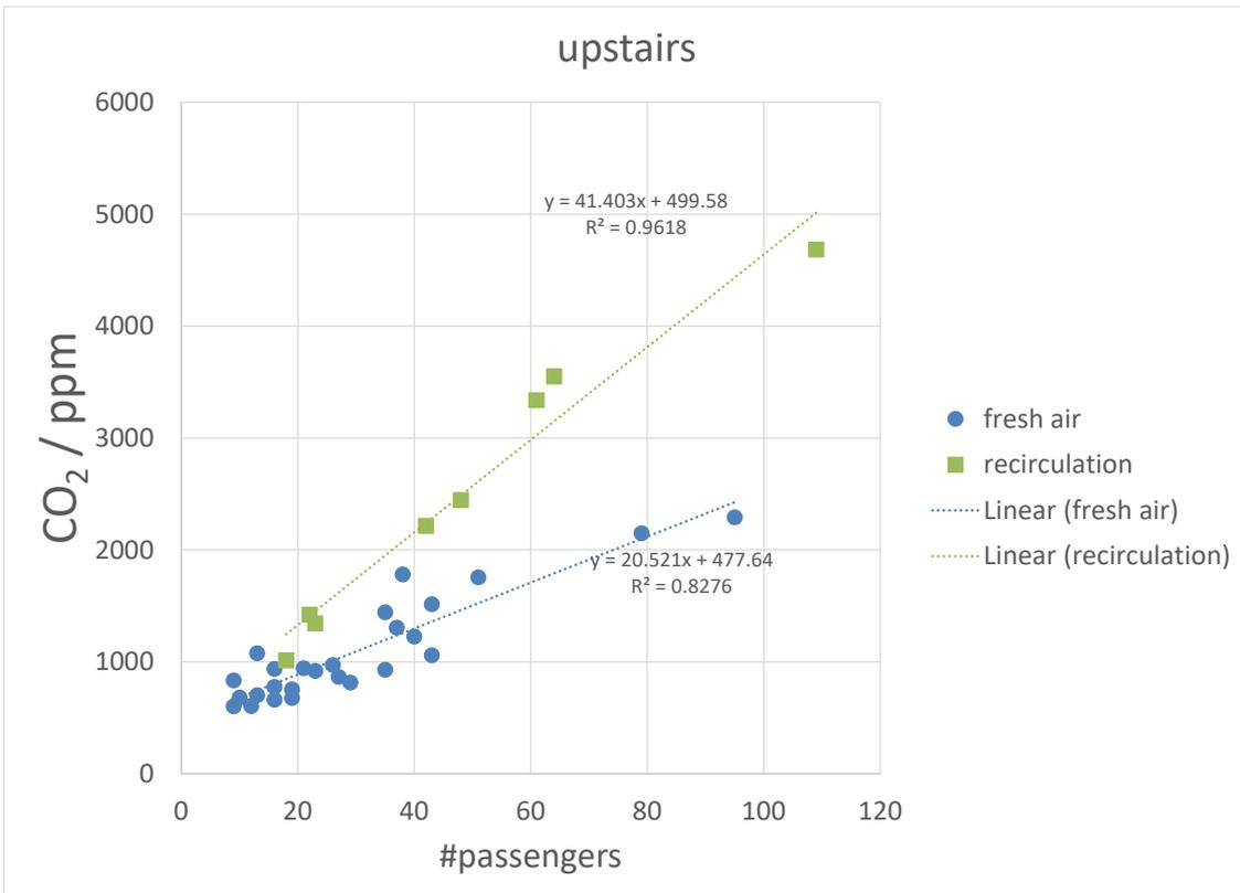
**Figure 3: Relationship between maximum CO<sub>2</sub> concentration on the upper deck and maximum number of passengers for each service run.**
