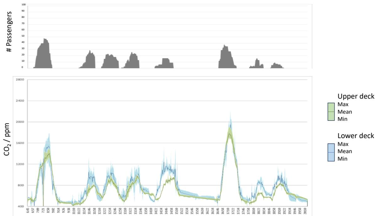
**Figure A-3: CO<sub>2</sub> and number of passengers on 13<sup>th</sup> April 2023 (fresh air).** Passenger numbers are likely in error from approx. 13:30 to 14:30.
