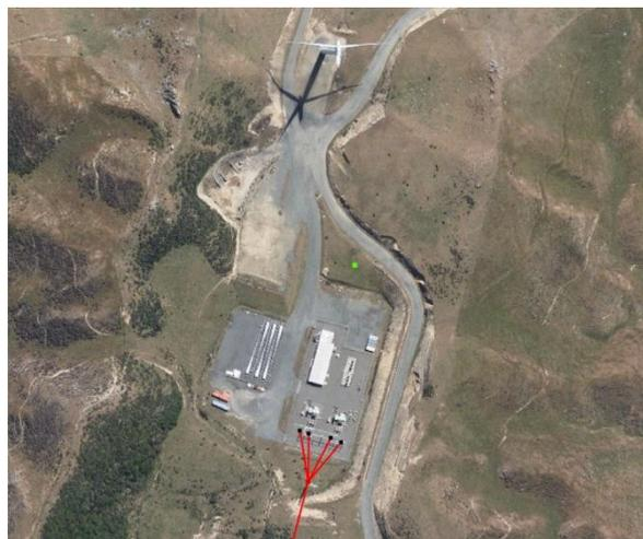
Figure 3: West Wind substation, located in the hills to the west of Mākara, takes electricity generated from the wind turbines at West Wind.
