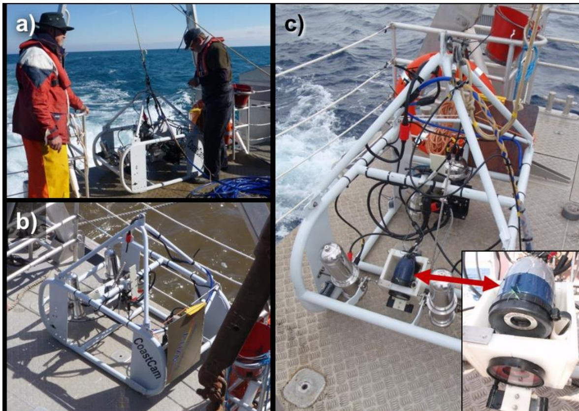
**Figure 2-5: NIWA CoastCam imaging system used to survey soft sediment habitats in Lyall Bay.**
