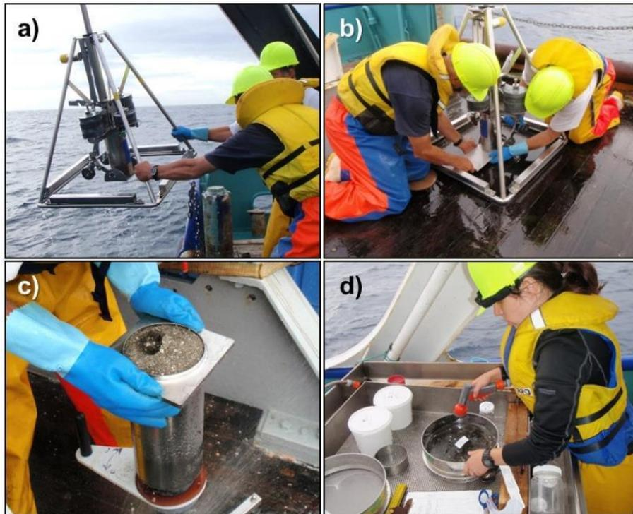
**Figure 2-9: Sediment and infaunal sampling using NIWA's KC Denmark HAPS corer.**
