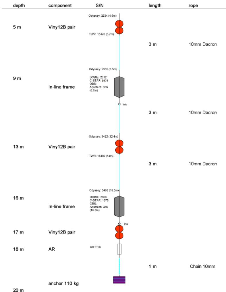
**Figure 2-2: The optical mooring design.** This diagram illustrates the positions (depths) of optical water quality sensors. S/N = serial number.
