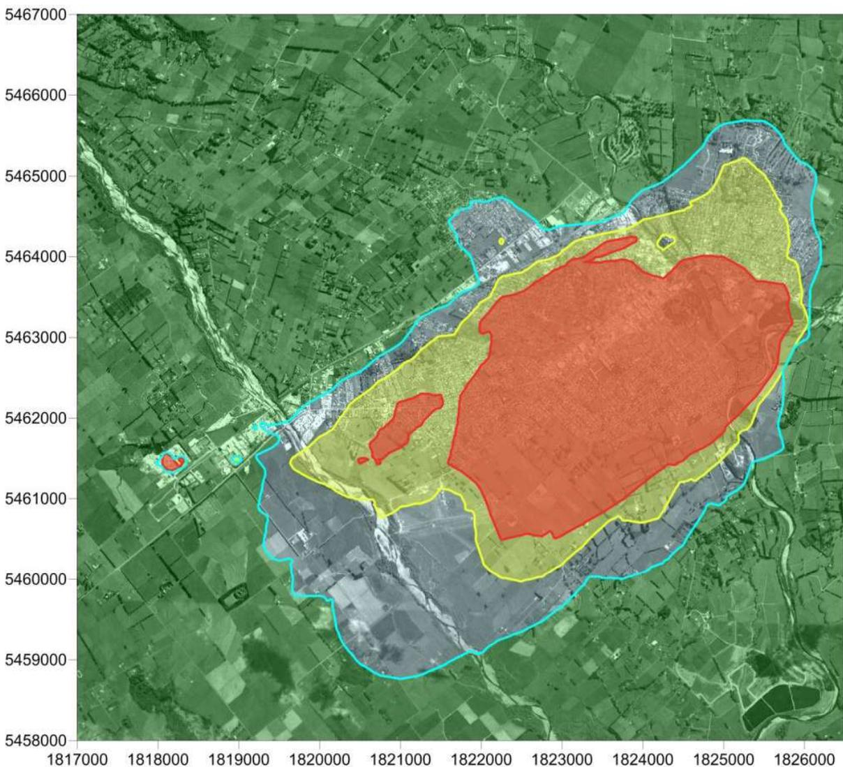
Figure 8: Airshed boundary around Masterton based on all years of modelling. Modelled boundary is in yellow; outer and inner boundaries accounting for modelling uncertainties are in blue and red, respectively.
